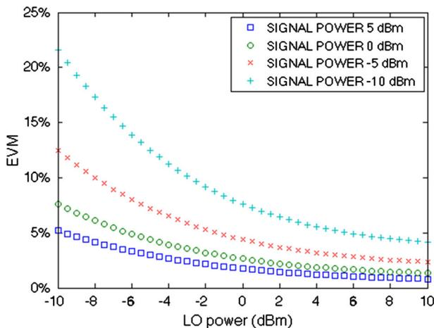
Fig. 5 EVM as a function of the local oscillator power, for various values of the signal power
