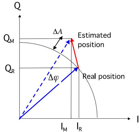
where  $(I_M - I_R)$  and  $(Q_M - Q_R)$  are the differences between the measured values, denoted with the subscript  $M$  and the actual values, denoted with the subscript  $R$ , for the two quadratures  $I$  and  $Q$  of the measured signal vector, respectively.
