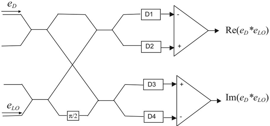
**Fig. 2** The double balanced homodyne detection (DBHD) arrangement
