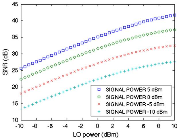
Fig. 4 Signal-to-noise ratio, as a function of the local oscillator power, for various values of the signal under test power
