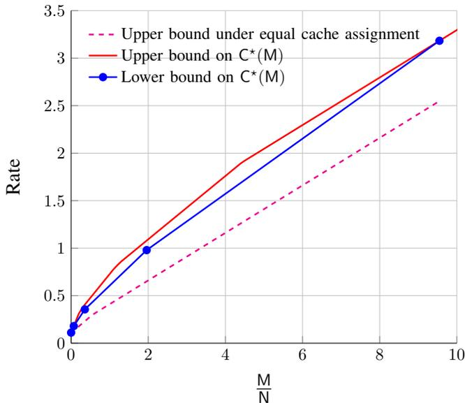
Fig. 5. Upper and lower bounds on  $C^*(M)$  on a 4-receiver Gaussian BC with input power  $P = 1$  and noise variances  $\sigma_1^2 = 4$ ,  $\sigma_2^2 = 1$ ,  $\sigma_3^2 = 0.5$ , and  $\sigma_4^2 = 0.1$ . We have  $N = 10$ .
