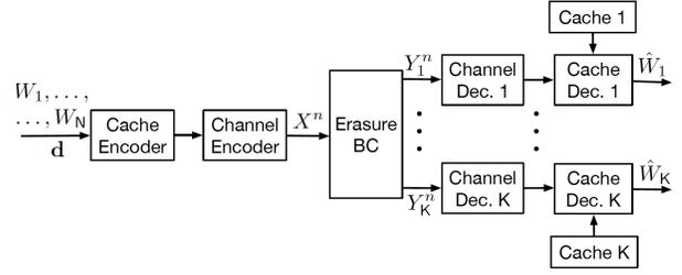
Fig. 2. Separate cache-channel coding architecture.
