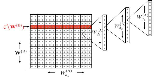
Fig. 3. Superposition piggyback code construction  $\mathcal{C}$  for  $K = 4$  receivers. Recall that receiver 1 is the weakest. Each dot represents a codeword.
