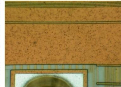
Nothing can be seen under the top metal layer on Microchip PIC16F877A microcontroller [37] as the layers inside the chip were planarised during fabrication. 500x magnification
