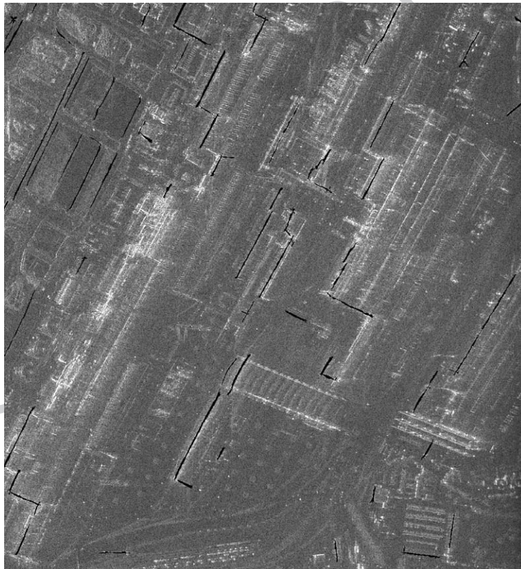
Fig. 5. Detection of the brightest linear features (black lines) in the SAR data.
