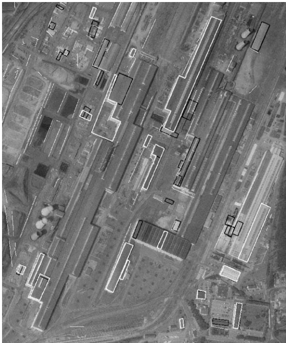
Fig. 11. Result of the automatic building detection: black and white polygons show objects detected by the rectangular box approach and the corner search tree, respectively, and white lines show SAR primitives.
