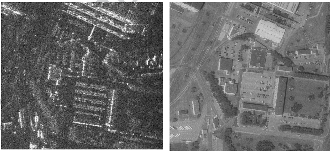
Fig. 1. Examples of the building appearance in the slant range SAR image with sensor viewing from the left (left) and the corresponding optical image (right).
