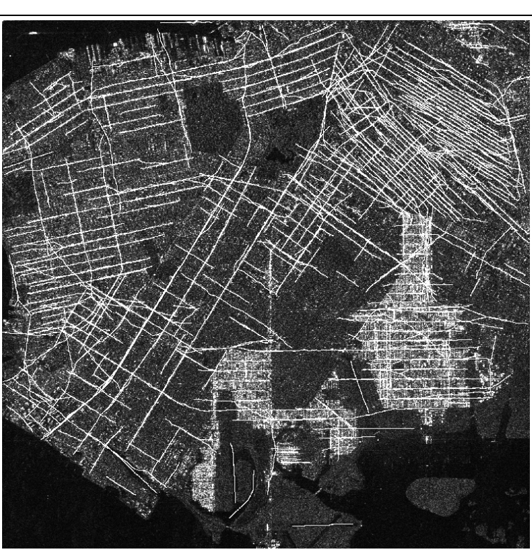
Figure 3: Automatic extraction of the road network (using one view)
