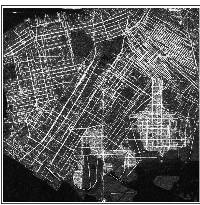
Figure 4: Automatic extraction of the road network using two views: the networks extracted on each view are superimposed.
