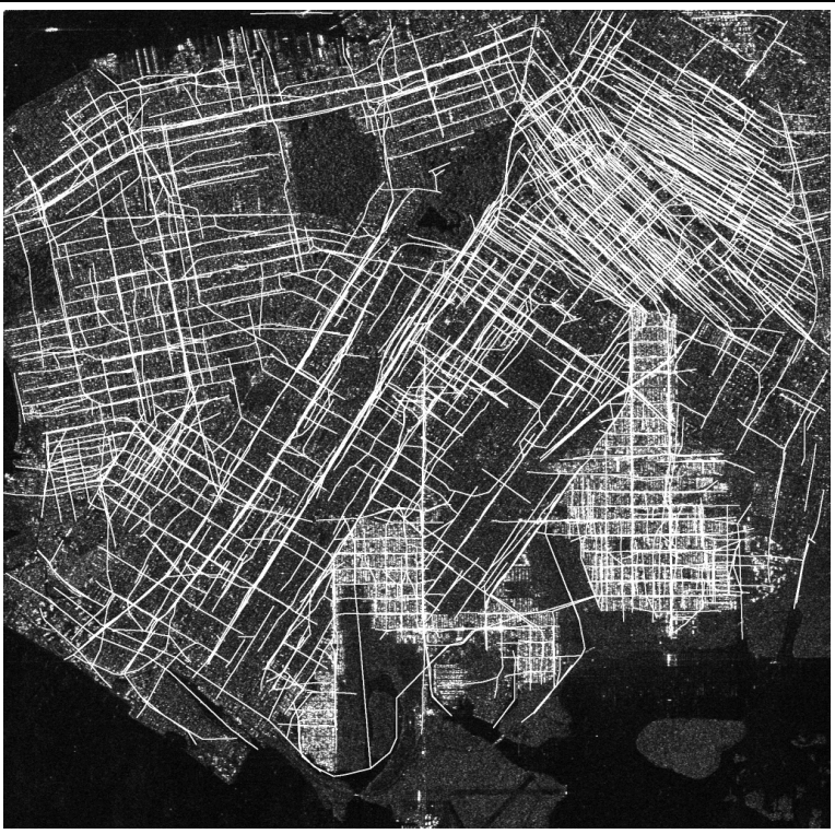
Figure 5: Automatic extraction of the road network using two views: the network is directly extracted using the 2 SAR images in the detection process.
