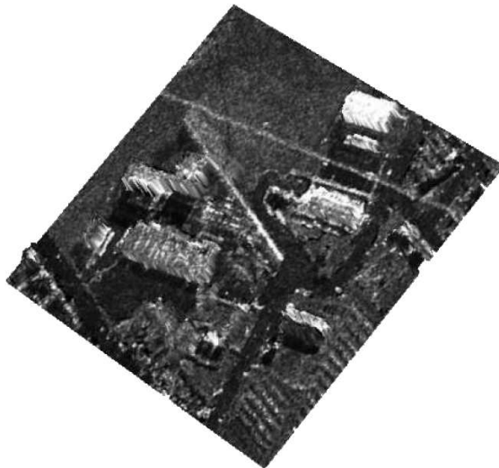
Fig. 6. Example of 3D reconstruction using the regularized interferometric phase with a joint prior with amplitude data, and graph-cut optimization (from [28]). The amplitude image is superimposed on the computed elevation (images acquired by ONERA).
