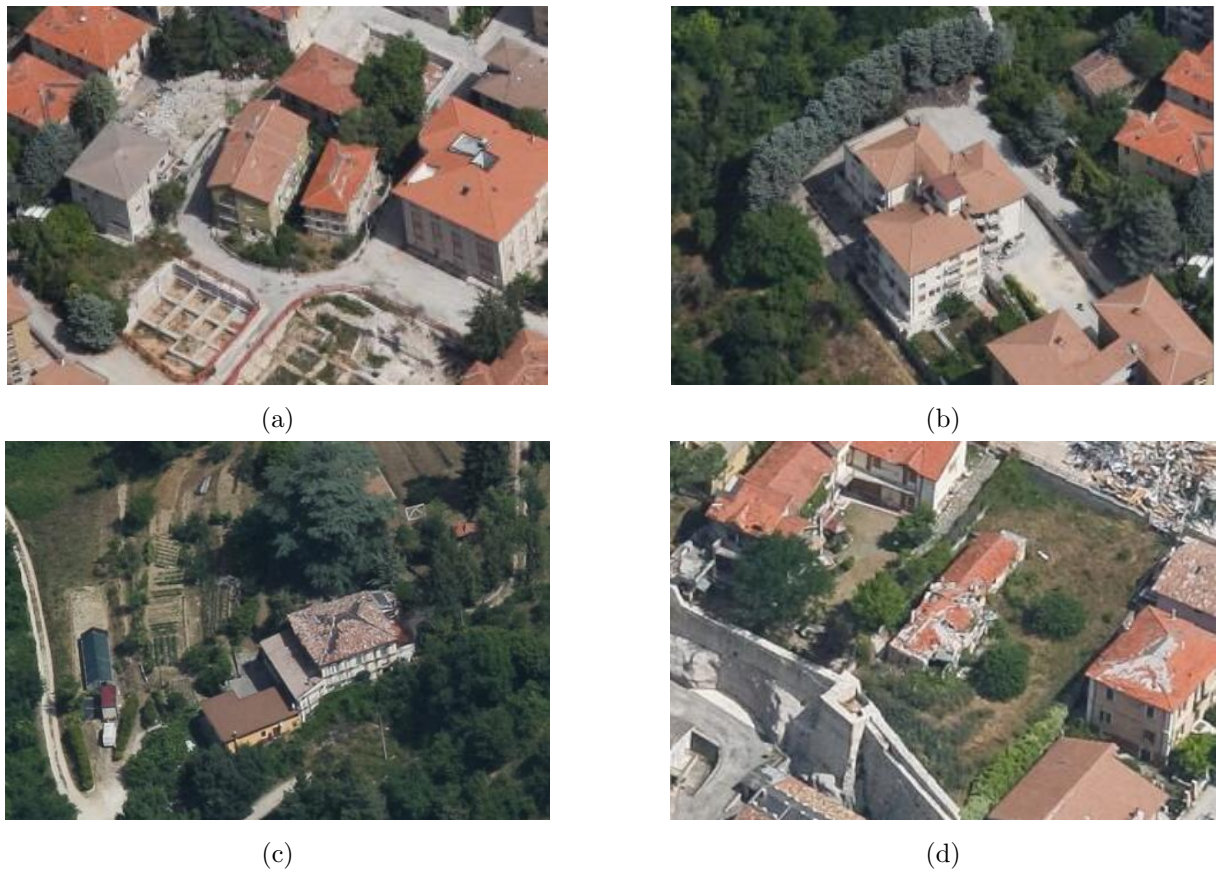
Figure 6.13: Crop 1: Examples for buildings detected by the proposed approach: a) miss (above) and correct (below) detection for Fully Destroyed building class; b) correct detection for Partially Destroyed Building class; c) false alarm for Partially Destroyed Building class; d) miss detection for Partially Destroyed Building class.
