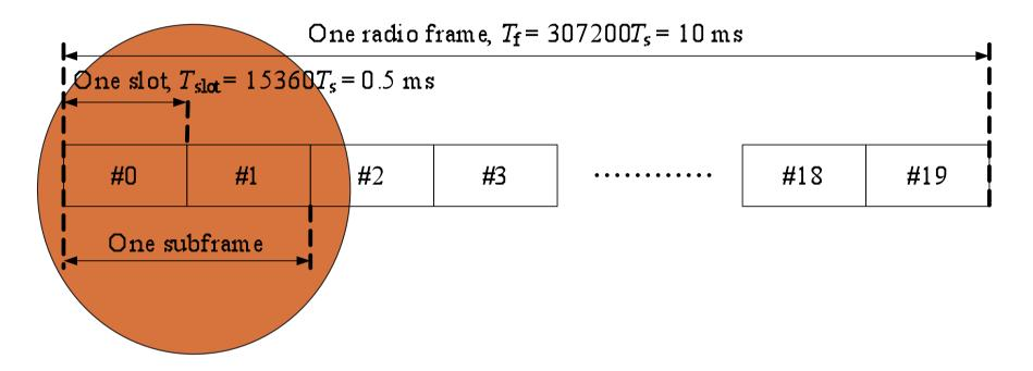
Granularity window of PHY control (1ms) => complete demodulation Sequence can be changed on this timescale -> tight RT constraints on OS and Inter-IP communication (10ms in UMTS, 5 ms in WIMAX)
