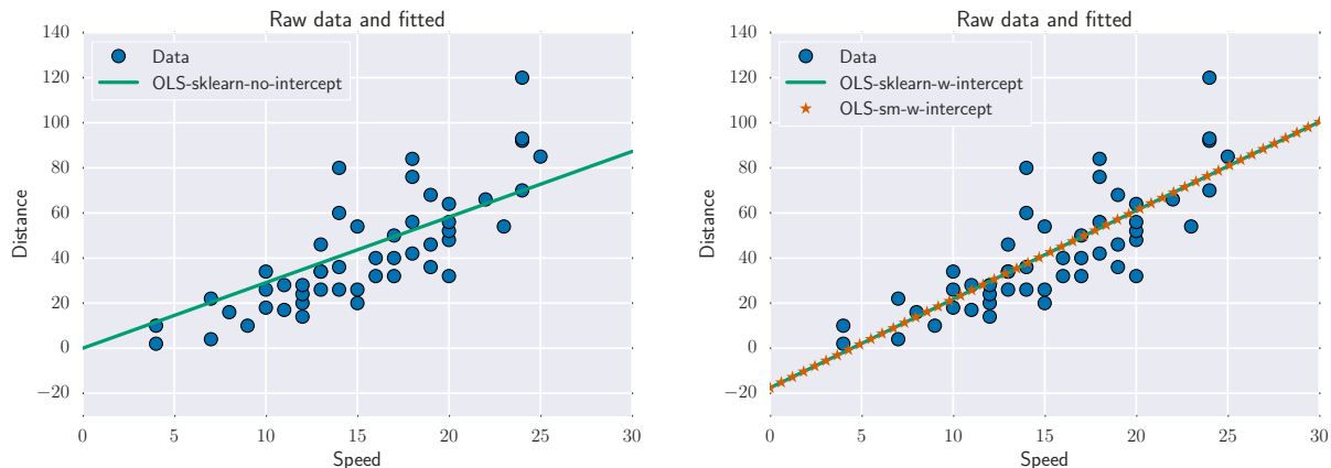
Figure 1.1: The dataset is the cars dataset from the R software. We use sklearn to compute OLS. The graph on the left represents the OLS line without intercept and the graph on the right is the OLS line computed with intercept.
