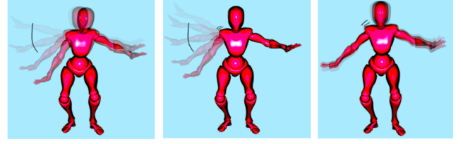
Figure 4: Effect of circumfixing lines on motion propagation. Left: Without circumfixing lines, the arm motion propagates to the entire upper body. Middle: Circumfixing lines over the shoulders constrain the motion, limiting it to the arm only. Right: With only circumfixing lines and no trajectory lines, the upper body exhibits a "shaking" motion.
