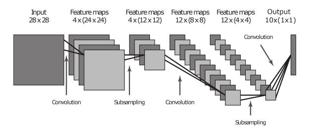
During each convolution use a  $5 \times 5$  kernel and  $2 \times 2$  kernel during each pooling. Use the rectified linear unit ('relu') as the activation function of the feature maps and tensorflow.keras.losses.SparseCategoricalCrossentropy as the loss.
