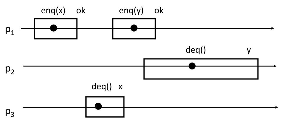
p<sub>1</sub>-enq(x); p<sub>1</sub>-ok; p<sub>3</sub>-deq(); p<sub>3</sub>-x; p<sub>1</sub>-enq(y); p<sub>1</sub> -ok; p<sub>2</sub>-dequeue(); p<sub>2</sub>-y
