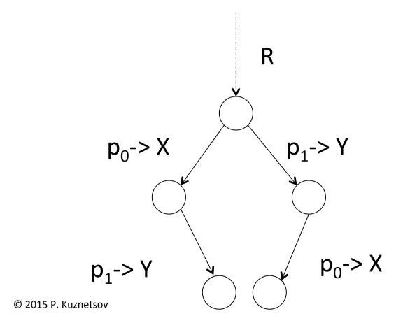
p<sub>0</sub> and p<sub>1</sub> are about to read the same object X
