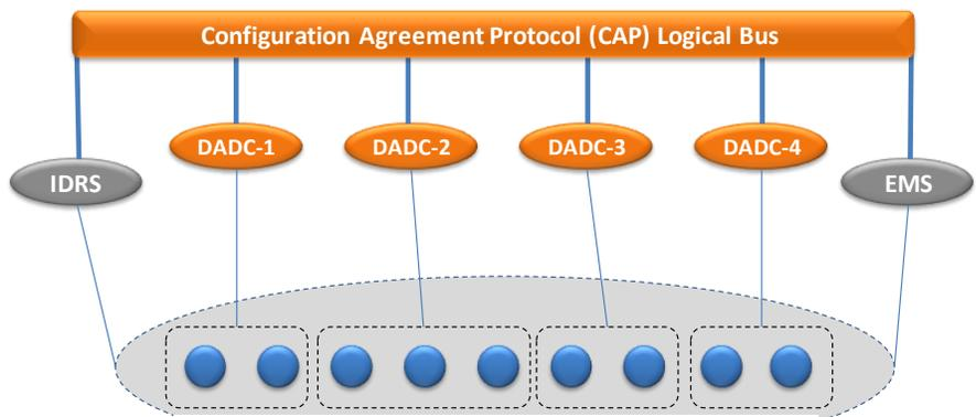
**Figure 2: Distributed ADC system architecture**
