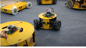
Fig 2. Omni-wheel XY motion capable Nexus robots
