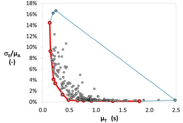
**Figure 6. Extracting the convex front of performance from pooled data. The data points of the convex hull are circled. The subset of them that form the critical South-West quadrant are connected with thicker line segments.**
