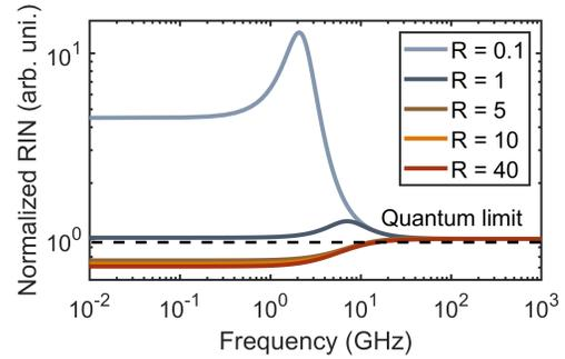
Fig. 3. Calculated normalized relative intensity noise spectra under different normalized noise-suppressed pump level  $R$ .
