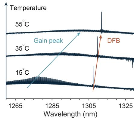
Fig. 1. (a) Optical spectra at  $2 \times I_{th}$  under different temperatures. The variations of gain peak and DFB peak are marked by the jade and the burgundy lines, respectively.
