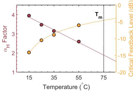
Fig. 2. Linewidth enhancement factor (red) and critical feedback level (yellow) at  $6 \times I_{th}$  as a function of the temperature. The optimum operating temperature at 75°C is marked by the dotted black line.
