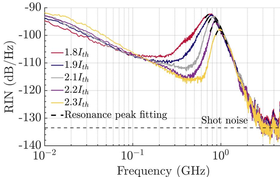
Figure 1. RIN spectrum measured over the 10 MHz-5 GHz interval at room temperature and for various pump currents. The horizontal dashed line represents the shot noise limit.
