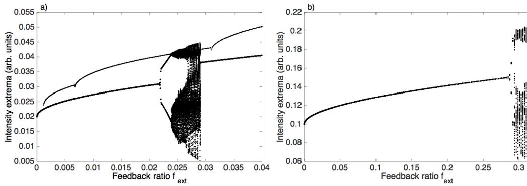
**Figure 3.** Influence of the bias parameter  $P$  on the bifurcation diagram for  $L_{ext} = 35$  cm and  $\alpha = 1.7$ . a) Numerical bifurcation diagram for  $P = 0.02$ . b) Numerical bifurcation diagram for  $P = 0.10$ .
