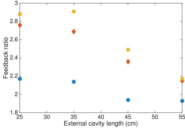
**Figure 4.** Influence of the external cavity length  $L_{ext}$  on the bifurcation diagram for  $P = 0.02$  and  $\alpha = 1.7$ . In blue circles, occurrence of the first Hopf bifurcation. In red diamonds, appearance of the LFF. In yellow squares, restabilization.
