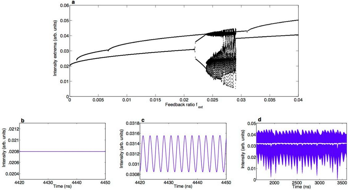
**Figure 1.** Numerical bifurcation diagram for  $P = 0.02$  and  $L_{ext} = 35$  cm, and associated time series. a) Numerical bifurcation diagram. b) Time trace for  $f_{ext} = 0.11\%$ , showing stable signal. c) Time trace for  $f_{ext} = 2.14\%$ , showing oscillations at the external cavity frequency. d) Time trace for  $f_{ext} = 2.59\%$ , showing both LFF and oscillations at the external cavity frequency.
