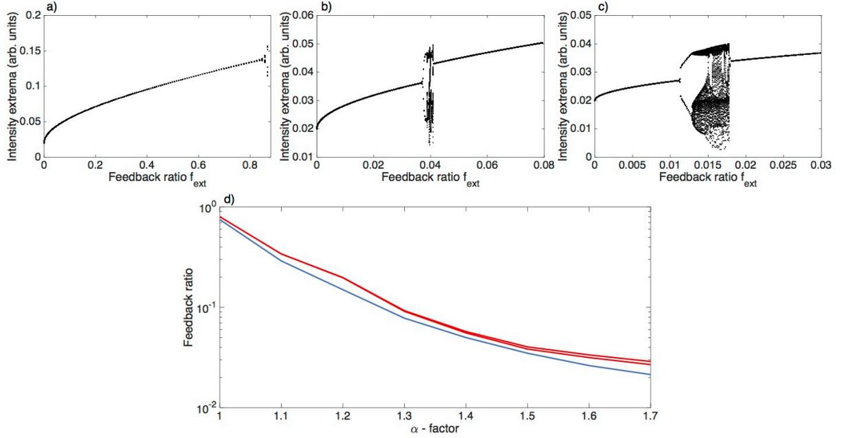
**Figure 2.** Influence of the  $\alpha$ -factor on the bifurcation diagram for  $P = 0.02$  and  $L_{ext} = 35$  cm. a) Numerical bifurcation diagram for  $\alpha = 1$ . b) Numerical bifurcation diagram for  $\alpha = 1.5$ . c) Numerical bifurcation diagram for  $\alpha = 2$ . d) Evolution of the Hopf point (in blue) and of the lower and upper limits of the LFF area (in red) as a function of the  $\alpha$ -factor.
