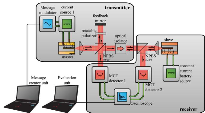
Fig. 1. Setup for chaotic secure communications with QCLs. The apparatus is split into two parts: one (with the master QCL) is dedicated to chaos masking and transmission whereas the other (with the slave QCL) is dedicated to synchronization and recovery. NPBS: non-polarizing beam-splitter, MCT: Mercury-Cadmium-Telluride.
