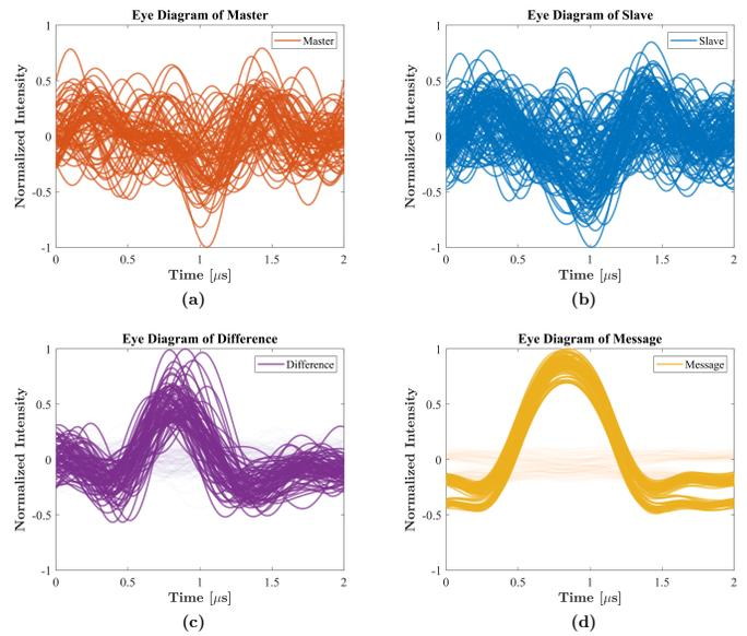
Fig. 3. Experimental eye diagrams for the 4 components of the previous figure. From these diagrams, one can see that it is impossible to recover the message only from the signal of the master QCL but it becomes possible for most of the bits from the difference signal. Bits deciphered as '0' are drawn with a light color while bits deciphered as '1' are drawn with a stressed color.
