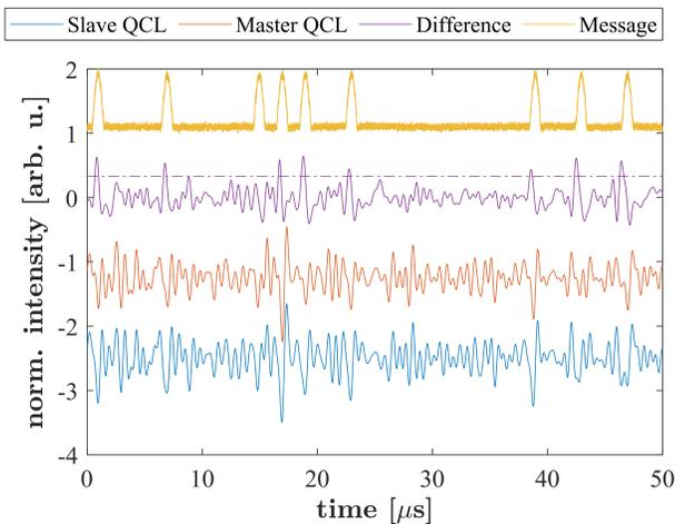
Fig. 2. Recovery process to decode the enciphered message. The blue curve is the filtered intensity of the slave QCL. The red curve is the filtered intensity of the master QCL. The violet curve represents the subtraction between the red curve and the blue curve and the dash-dotted line corresponds to the threshold used to detect a '1'-bit. The orange curve is the magnified initial message, subsequently hidden within the red curve.
