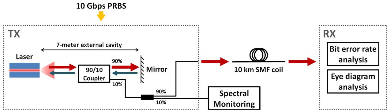
Figure 2. Experimental set-up used for optical feedback investigation.
