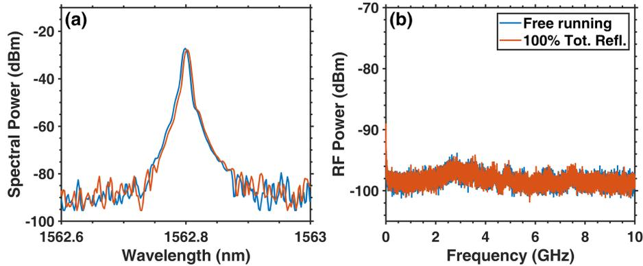
Figure 3. (a) Optical and (b) RF spectra of the high- $Q$  DFB laser biased at  $3 \times I_{th}$  for the free-running case (blue) and under 100% (i.e., -14 dB) optical feedback (red) at  $T = 20^\circ\text{C}$ .
