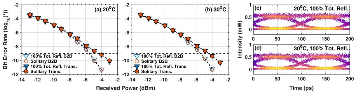
Figure 5. BER characteristics of the high- $Q$  laser at (a)  $T = 20^\circ\text{C}$  and (b)  $T = 30^\circ\text{C}$  with (hollow and solid blue triangles) and without (hollow and solid orange circles) feedback; eye diagrams with maximal feedback after transmission over 10 km fiber coil at (c)  $T = 20^\circ\text{C}$  and (d)  $T = 30^\circ\text{C}$ .
