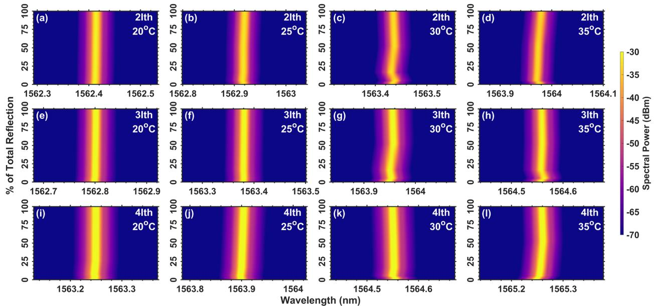
Figure 4. Optical spectral maps of the high- $Q$  laser at  $T = 20^\circ\text{C}$ ,  $25^\circ\text{C}$ ,  $30^\circ\text{C}$ ,  $35^\circ\text{C}$  under 3 different bias conditions of  $I = 2 \times I_{th}$  ((a),(b),(c),(d)),  $3 \times I_{th}$  ((e),(f),(g),(h)) and  $4 \times I_{th}$  ((i),(j),(k),(l)).
