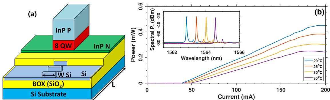
Figure 1. (a) Schematic of the high- $Q$  DFB laser structure; (b) L-I curves of high- $Q$  DFB laser at  $T = 20^\circ\text{C}$ ,  $25^\circ\text{C}$ ,  $30^\circ\text{C}$ , and  $35^\circ\text{C}$ ; the inset depicts the optical spectra under  $3 \times I_{th}$  at each temperature.
