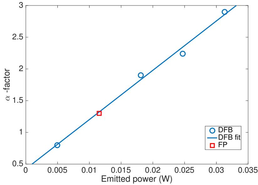
Figure 3. Evolution of the  $\alpha$ -factor with the laser output power. The blue circles correspond to the measurements on the DFB QCL with the self-mixing technique and the blue line to the linear fit of these results. The red square corresponds to the LEF measurement of the FP QCL using the wavelength shift with optical feedback.
