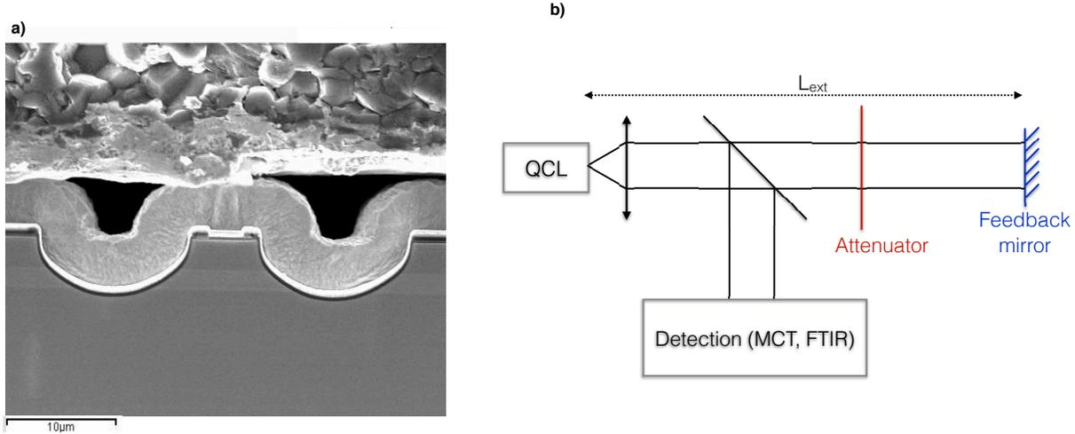
Figure 1. a) SEM picture of the QCL under study. The active area appears in lighter gray. b) Experimental setup.
