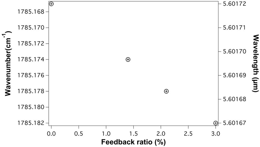
Figure 2. Evolution of the wavelength of one longitudinal mode of the FP spectrum under weak optical feedback.
