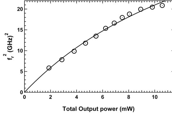
Fig. 3. The square of the resonance frequency versus the output power
