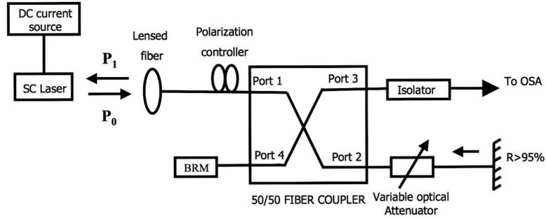
Fig.1. Schematics of the experimental apparatus for the feedback measurements.
