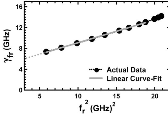
Fig. 4. The damping factor versus the square of the relaxation frequency
