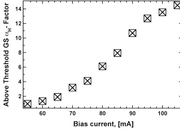
Fig. 5. The above threshold GS  $\alpha_H$ -factor versus the bias current.
