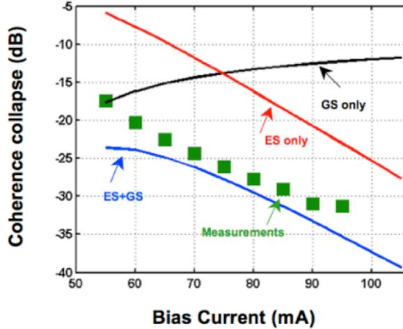
Fig. 7. Coherence collapse thresholds as a function of the bias current.
