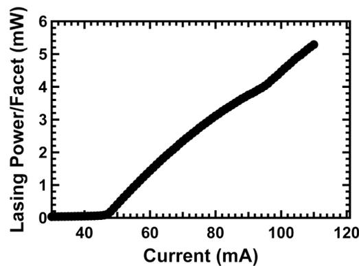
Fig.2. The light current characteristic of the QD laser under study.
