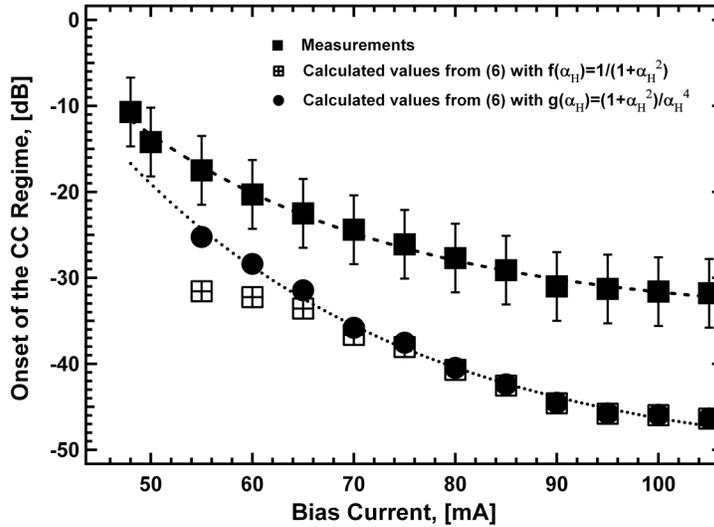
Fig. 6. Coherence collapse thresholds as a function of the bias current.
