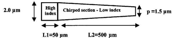
Fig. 1. Design of the device showing a 50- $\mu\text{m}$ -long straight section (high index) followed by a 500- $\mu\text{m}$ -long tapered stripe section (low index).
