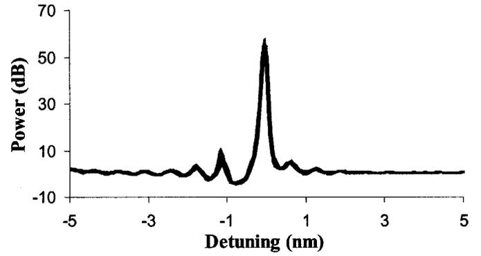
Fig. 3. Superimposition of twelve measured spectra at 10 mW versus the Bragg detuning. SMSR = 47 dB;  $\Delta\lambda = 1.1 \text{ nm}$ .
