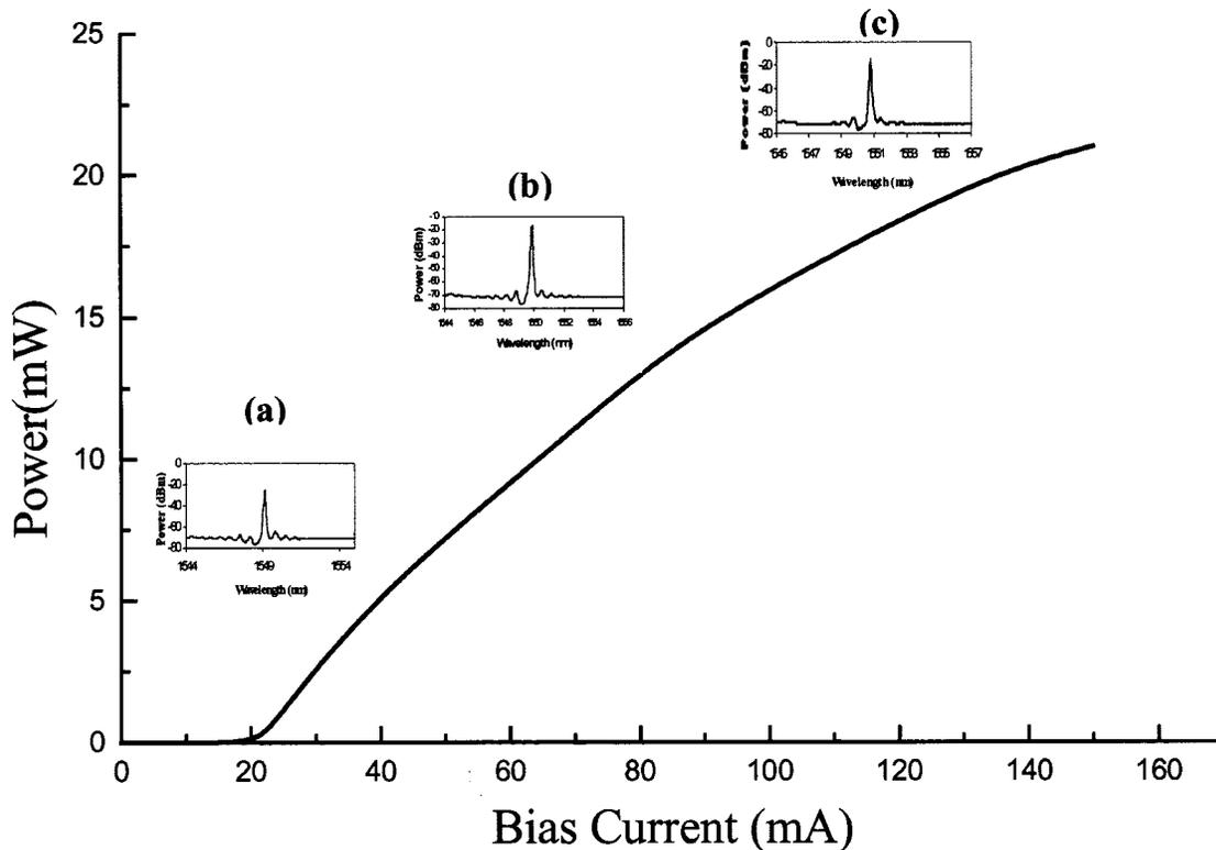
Fig. 5. Light current characteristic:  $I_{th} = 20$  mA,  $\eta = 0.26$  W/A. Inset: Spectra at different injected current. (a)  $I = 27$  mA SMSR = 39 dB. (b)  $I = 63$  mA SMSR = 47 dB. (c)  $I = 116$  mA SMSR = 51 dB.
