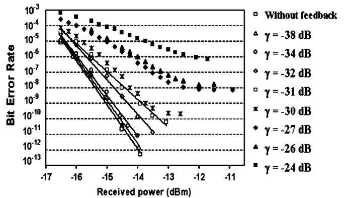
Fig. 6. BER versus received power for different feedback levels at 30 mA.
