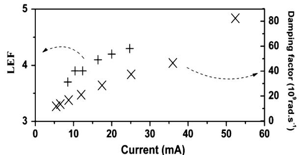
Fig. 2. LEF and damping factor versus current.
