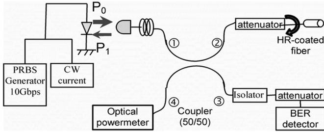
Fig. 3. Experimental setup for feedback tolerance measurements at 10 Gb/s.
