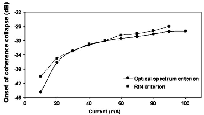
Fig. 5. Onset of coherence collapse (decibels) versus current.
