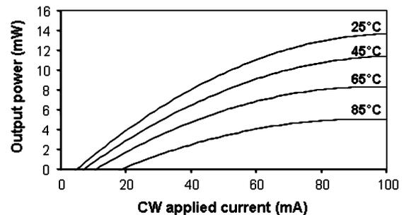
Fig. 1. Light-current characteristics at different temperature values.
