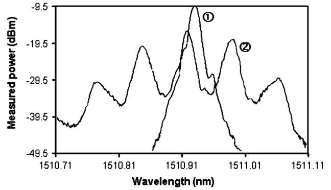
Fig. 4. Optical spectrum: (1) without optical feedback; (2) with optical feedback and beginning of coherence collapse.
