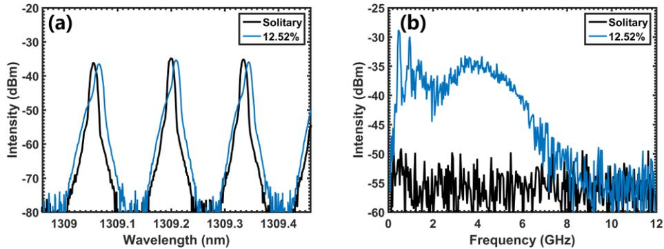
Figure 4. GS QD laser at a bias level of  $2.5 \times I_{\text{th}}$ : (a) optical and (b) electrical spectra of the free-running laser (0%) and maximal (12.52%) optical feedback.
