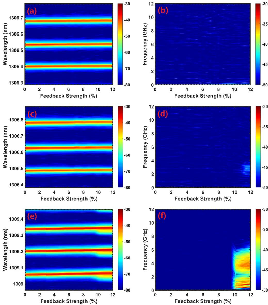
Figure 3. GS QD laser: optical spectra (a) and electrical spectra (b) mapped at  $1.5\times I_{th}$ , at  $2\times I_{th}$  (c), (d) and  $2.5\times I_{th}$  (e), (f).
