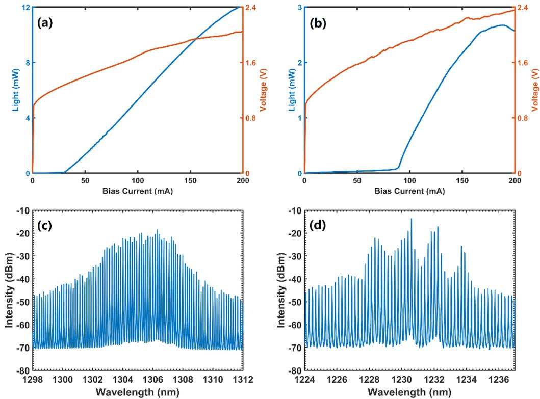
Figure 1. (a) LIV curves and (c) optical spectrum measured at  $2 \times I_{th}$  of the GS laser; (b) LIV curves and (d) optical spectrum measured at  $2 \times I_{th}$  of the ES laser. All measurements are performed at 20 °C.
