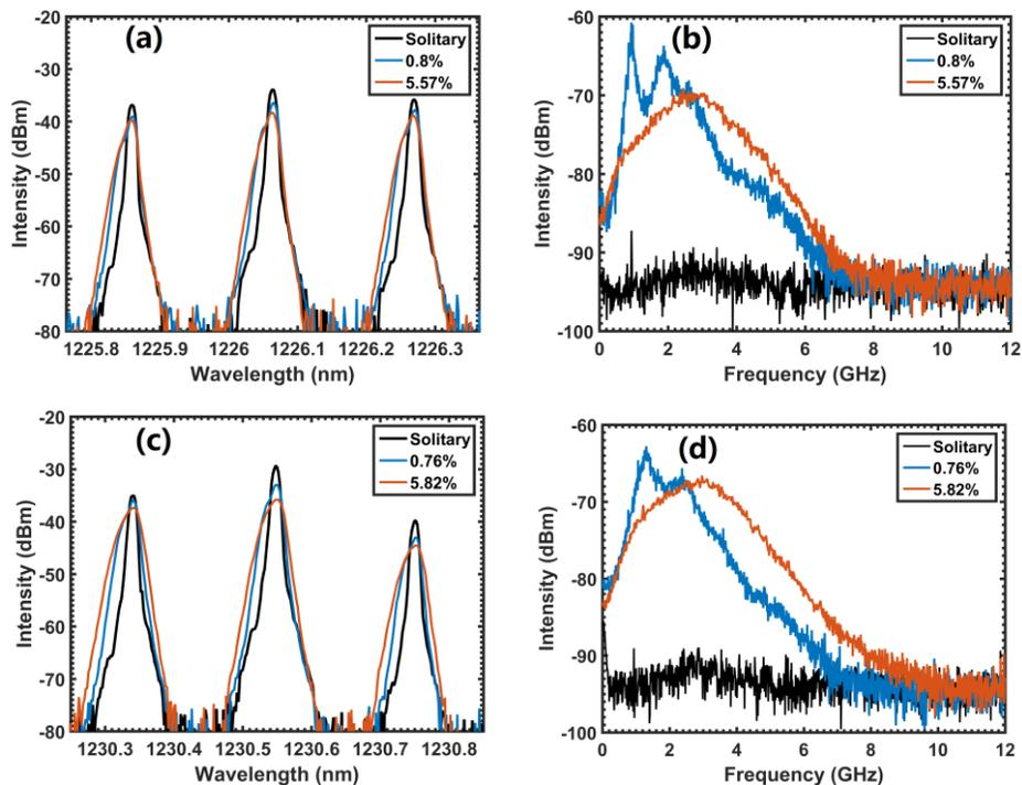
Figure 6. ES QD laser at  $1.5\times I_{th}$  bias level: (a) optical and (b) electrical spectra of the free-running laser, 0.8% and 5.57% optical feedback; ES laser at  $2\times I_{th}$  bias level: (c) optical and (d) electrical spectra of the free-running laser, 0.76% and 5.82% optical feedback.
