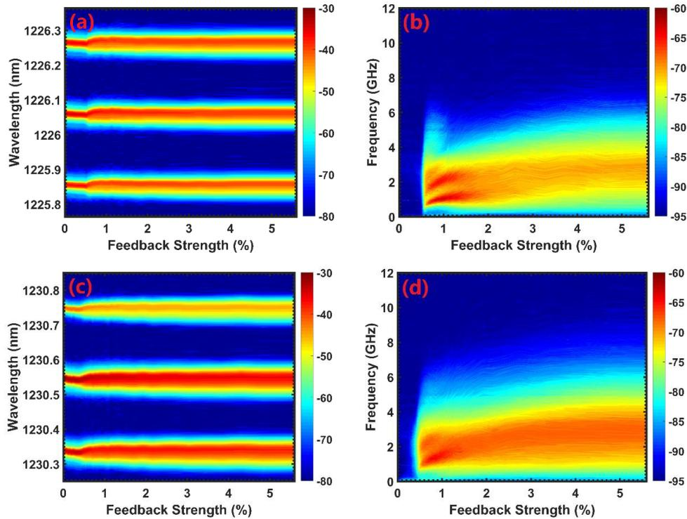
Figure 5. ES laser: optical spectra maps at (a)  $1.5 \times I_{\text{th}}$ , (c)  $2 \times I_{\text{th}}$ , and electrical spectra maps at (b)  $1.5 \times I_{\text{th}}$ , (d)  $2 \times I_{\text{th}}$ .
