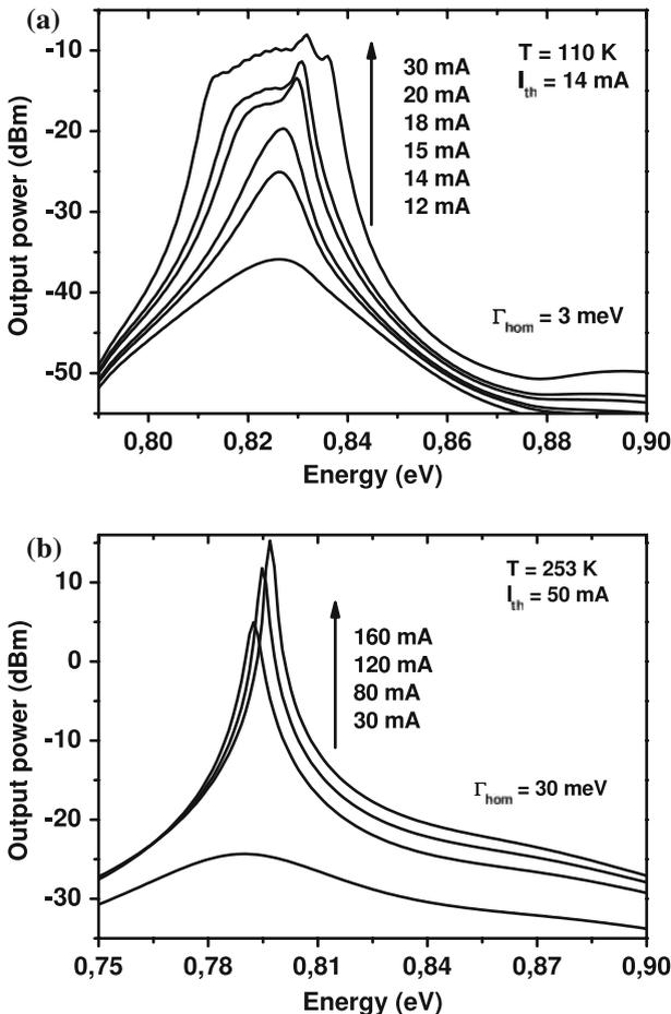
**Fig. 4** Calculated emission spectra of a semiconductor laser with a single QD layer on InP(311)B substrate for two different temperatures: (a) 110 K and (b) 253 K
