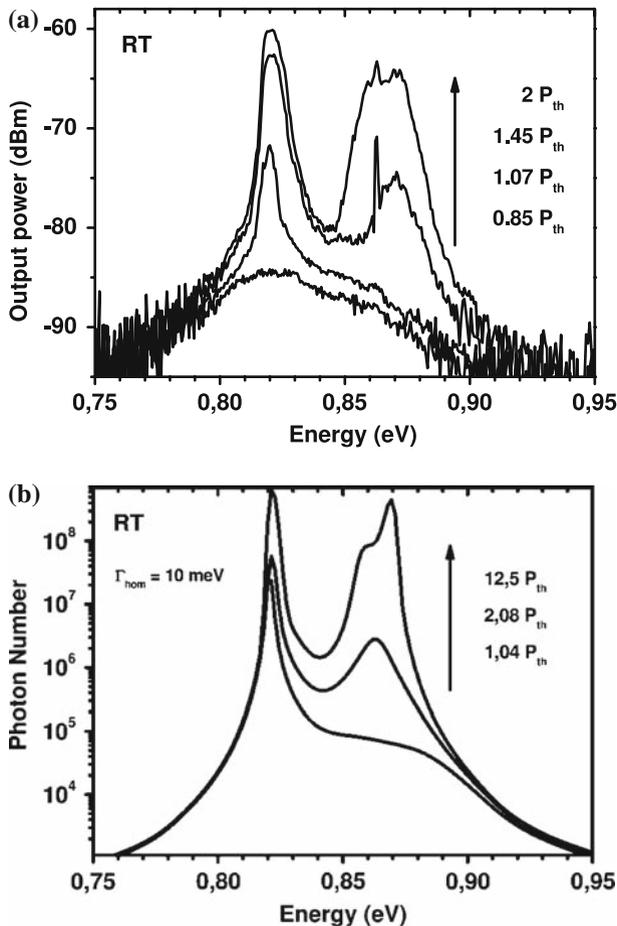
**Fig. 2** Room temperature emission spectra of a QD broad area laser with six QD stacked layers (undoped structure) under a pulsed optical excitation a) and simulated laser emission spectra for the same device at  $\Gamma_{\text{hom}} = 10 \text{ meV}$
