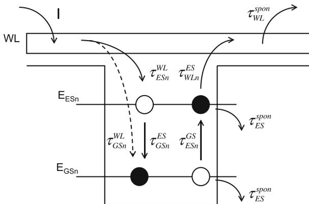
**Fig. 1** Schematic representation of the carrier dynamics model with direct relaxation channel (dash line) for the  $n$ -th QD sub-group
