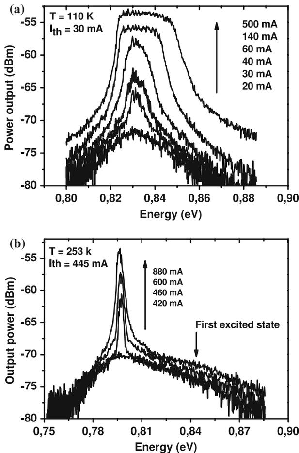
**Fig. 3** Lasing and electroluminescence spectra under pulsed injection mode for two different temperatures: (a) 110 K and (b) 253 K. At each temperature, spectra at several injection currents are displayed and the threshold current ( $I_{th}$ ) is given
