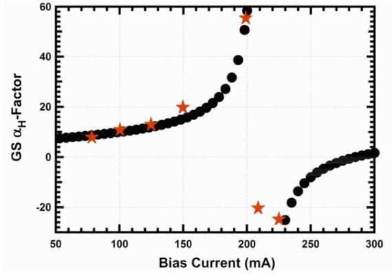
Fig. 6. Calculated GS  $\alpha_H$ -factor versus the bias current (black dots). Superimposed red stars correspond to experimental data from [23].
