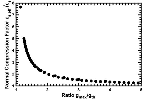
Fig. 2. Normalized compression factor as a function of  $g_{\text{max}}/g_{\text{th}}$ .
