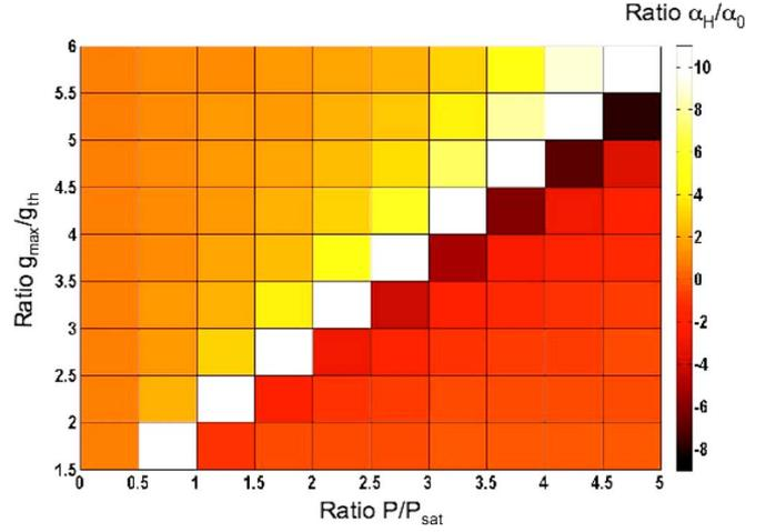
Fig. 5. Stability map based on the normalized linewidth-enhancement factor  $\alpha_H/\alpha_0$  in the  $(P/P_{\text{sat}}, g_{\text{max}}/g_{\text{th}})$  plane.
