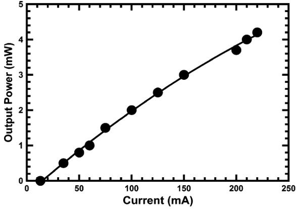
Fig. 1.  $L(I)$  characteristic of the InAs–GaAs QD laser under study. At room temperature, the threshold current for the GS is 13 mA and the external differential efficiency is about 0.02 W/A.
