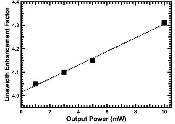
Fig. 4. Effective linewidth-enhancement factor  $\alpha_H$  as a function of the output power for the QW DFB laser.
