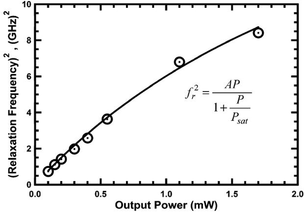
Fig. 3. Square of the resonance frequency versus the output power. The curve-fitting equation is shown in the inset and leads to  $A = 7.5 \pm 0.2$  (GHz)<sup>2</sup> mW<sup>-1</sup> and  $P_{\text{sat}} = 3.3 \pm 0.3$  mW.
