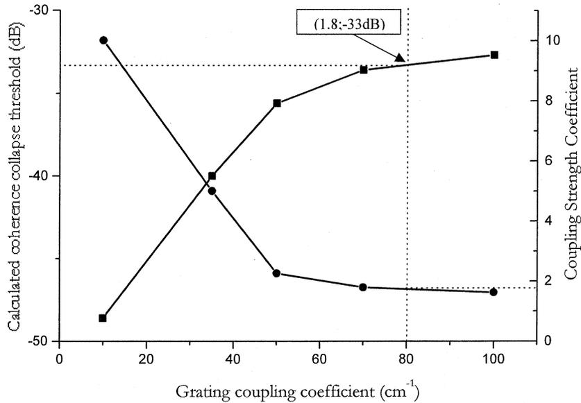
Fig. 10. Variations of the coupling strength coefficients (black dots) and of the coherence collapse threshold (black squares) versus the grating coupling coefficient for design (b).
