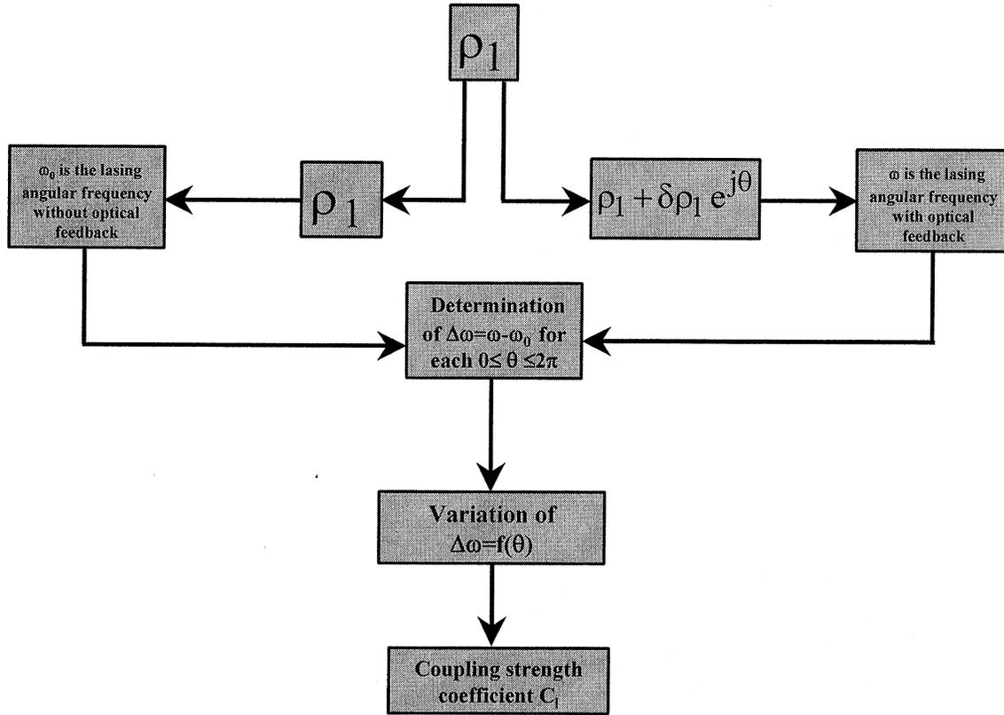
Fig. 1. Scheme of the algorithm used for the calculation of the coupling strength coefficient. The variation of the  $k$ -facet reflectivity subjected to the external reflection is done from  $\rho_k$  to  $\rho_k + \delta\rho_k e^{j\theta}$ . The knowledge of  $\omega_0$  and  $\omega(\theta)$  allows us to determinate explicitly the overall variation  $\Delta\omega(\theta) = \omega(\theta) - \omega_0$  as well as the coupling strength coefficient  $C_k$  through (15).
