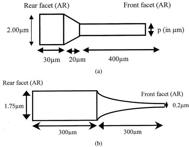
Fig. 6. Designs of the chirped-grating DFB lasers investigated with their different marks. They are made of a straight section followed by a varying width stripe section and have an AR coating on both facets so as to suppress facet phase effects. Design (a): the tip width  $p$  is in the range from 1.1 to 1.7  $\mu\text{m}$ . Design (b): the grating coupling coefficient is in the range from 10 to 100  $\text{cm}^{-1}$ .
