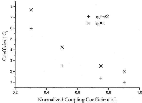
Fig. 3. Variations of the calculated coupling strength coefficient versus the normalized grating coupling coefficient ( $0.3 \leq \kappa L \leq 0.9$ ) for a 350- $\mu\text{m}$  AR/HR conventional DFB laser. The phase of the HR facet  $\varphi_r$  is fixed either to  $\pi/2$  (+ points) or  $\pi$  (x points).
