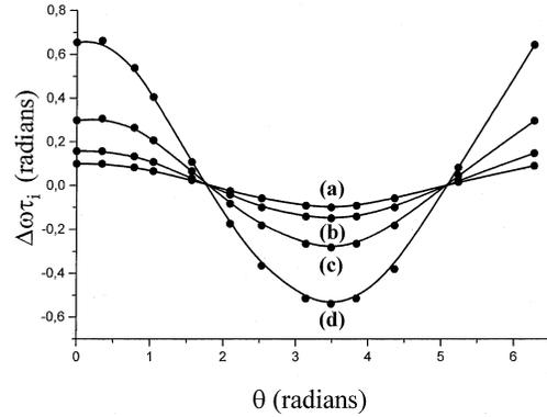
Fig. 4. Variations of the calculated normalized laser angular frequency  $\Delta\omega\tau_i$  versus the phase  $\theta$  for a 350- $\mu\text{m}$  AR/HR conventional DFB laser and for different normalized grating coupling coefficients  $\kappa L$ : (a)  $\kappa L = 0.3$ , (b)  $\kappa L = 0.5$ , (c)  $\kappa L = 0.7$ , and (d)  $\kappa L = 0.9$ .
