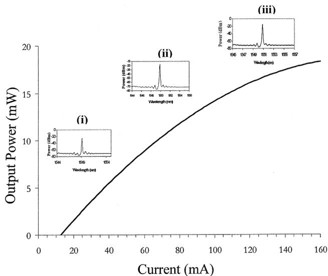
Fig. 7. Light-current characteristic relative to design (a) in Fig. 6. Threshold current at 25  $^{\circ}\text{C}$ :  $I_{\text{th}} = 12$  mA, External efficiency at 25  $^{\circ}\text{C}$ :  $\eta = 0.19$  W/A. Experimental optical spectra recorded at 3 mW (i), 6 mW (ii), and 15 mW (iii) are reported in the inset.
