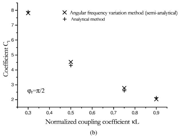
Fig. 5. Variations of the coupling strength coefficients  $C_l$  versus the normalized grating coupling coefficient calculated either with the analytical method (+ points) or with the method of the angular frequency variation (x points). The laser is a 350- $\mu\text{m}$  AR/HR conventional DFB. Two facet phase cases  $\varphi_r$  are investigated: (a)  $\varphi_r = \pi$  and (b)  $\varphi_r = \pi/2$ .
