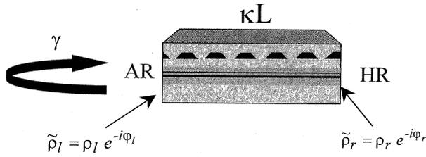
Fig. 2. Design of the AR/HR straight-section studied laser. The amount  $\gamma$  denotes the optical feedback reinjected into the cavity through the left facet and  $\kappa L$  is the normalized coupling coefficient.  $\tilde{\rho}_l$  and  $\tilde{\rho}_r$  correspond to the complex amplitude reflectivities on the AR and HR facets, respectively.
