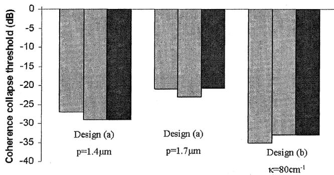
Fig. 11. Comparison between measured (in gray) and calculated (in black) coherence collapse thresholds  $\gamma_C$ . Design (a):  $p = 1.4 \mu\text{m}$ ,  $\gamma_C = -28$  dB (for a prediction of  $-29.1$  dB). Design (a):  $p = 1.7 \mu\text{m}$ ,  $\gamma_C = -22$  dB (for a prediction of  $-20.7$  dB). Design (b):  $\gamma_C = -34$  dB (for a prediction of  $-33$  dB).
