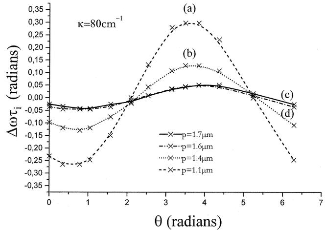
Fig. 8. Variations of the calculated normalized laser angular frequency  $\Delta\omega\tau_i$  versus the phase  $\theta$  for design (a). The grating coupling coefficient is equal to 80  $\text{cm}^{-1}$ . Simulations are conducted for the following values of the parameter  $p$ : (a)  $p = 1.1$   $\mu\text{m}$ , (b)  $p = 1.4$   $\mu\text{m}$ , (c)  $p = 1.6$   $\mu\text{m}$ , and (d)  $p = 1.7$   $\mu\text{m}$ .
