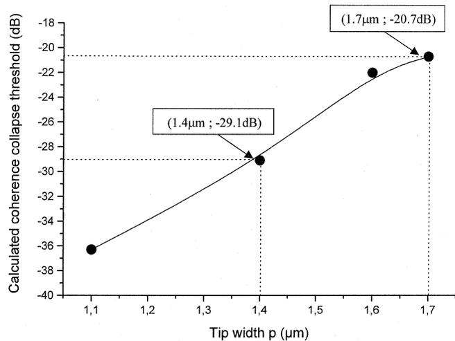
Fig. 9. Variations of the calculated coherence collapse threshold versus the tip width for design (a). Each point corresponds to a calculated value whereas a fit has been added to improve clarity.
