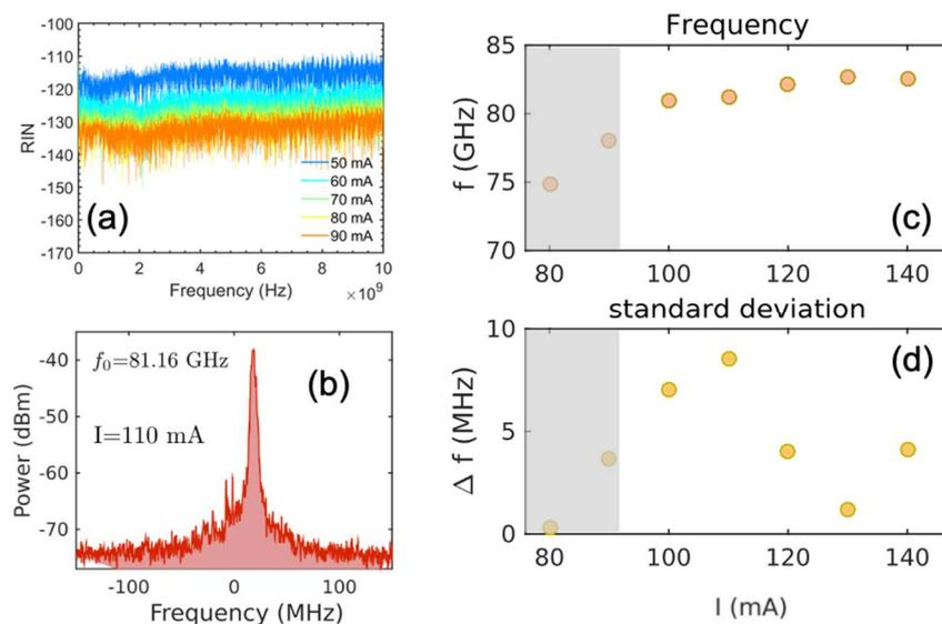
Fig. 1 (a) The relative intensity noise (RIN) captured at different bias currents; (b) The radiofrequency (RF) beatnote at 80 GHz measured at 110 mA. The linewidth is measured at 500 kHz; (c) Measured tunability of the RF beatnote with respect to the bias current; (d) Corresponding standard deviation with respect to the bias current.
