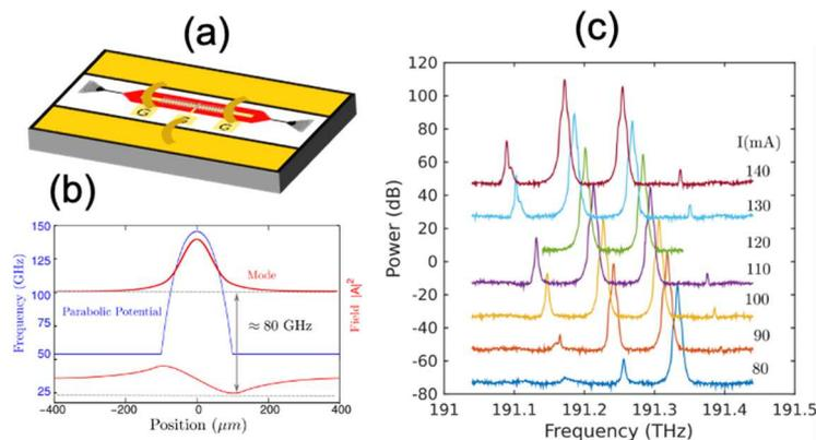
Fig. 1 (a) Schematic of the tapered DFB cavity; (b) band structure showing the offset frequency of 80 GHz (c) Measured optical spectra at different bias current conditions.
