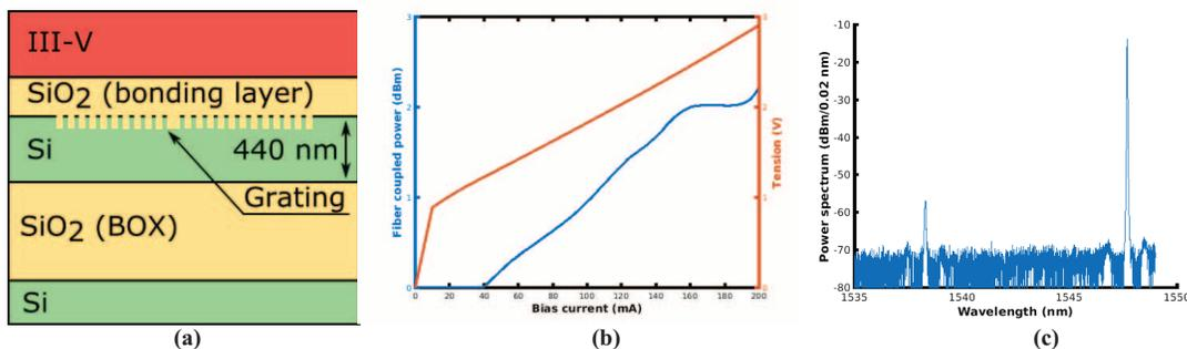
Fig. 1: (a) Cross section of the device. (b) Laser L-I-V curve. (c) optical spectrum at 110 mA showing SMSR superior to 40dB
