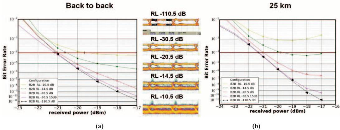
Fig. 3: BER measurements at 2.5 Gb/s (a): back to back and (b) after 25km transmission. Back to back eye diagrams are also shown.
