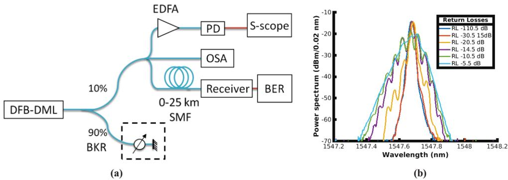
Fig. 2: (a) Experimental set-up showing the feedback module and the receiver side. (b) Spectrum for different return losses showing spectrum enlargement due to self sustained relaxation oscillation.
