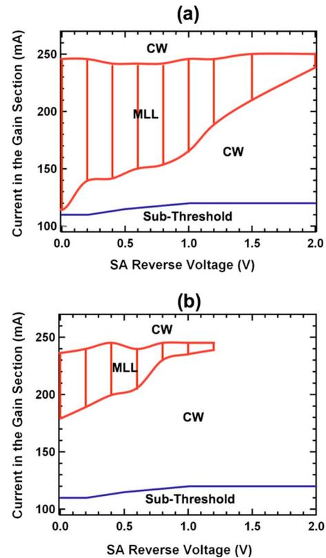
FIG. 2. (Color online) An operational map for combinations of the gain current and the SA reverse voltage. The ML condition is represented through the red dashed area. Subthreshold and cw regions are visible in between (a) without external optical feedback and (b) under maximum optical feedback ( $\Gamma = -24$  dB).
