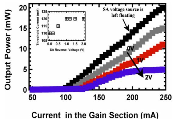
FIG. 1. (Color online) Light current characteristics measured at room temperature for different conditions: SA voltage source is left floating (black) and for SA reverse voltages of 0 V (gray), 1 V (red), and 2 V (blue). The figure in inset shows the threshold current as a function of the SA reverse voltage.
