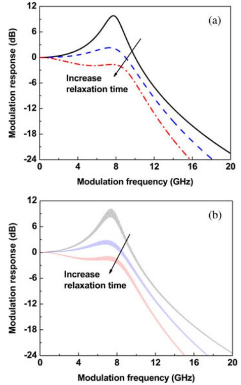
Fig. 9. Impacts of various carrier relaxation time  $0.2 \tau_{\text{GS}}^{\text{ES}}$ ,  $1.0 \tau_{\text{GS}}^{\text{ES}}$ , and  $2.0 \tau_{\text{GS}}^{\text{ES}}$  on the IM response for (a) short external cavity ( $f_{\text{ext}} = 10^{-3}$ , LEF = 1) and (b) long external cavity ( $f_{\text{ext}} = 10^{-5}$ , LEF = 5).
