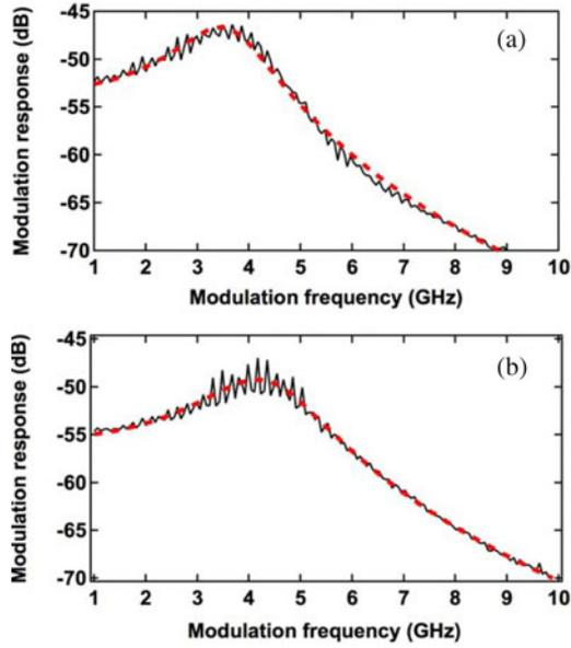
Fig. 5. Impacts of optical feedback ( $f_{\text{ext}} = 10^{-3}$ ) on the IM response of a 1.55- $\mu\text{m}$  InAs/InP QD laser operating under a long external cavity at different pump current (a) 75 mA and (b) 115 mA. In both cases, red-dashed lines correspond to the free-running curve-fitting functions.
