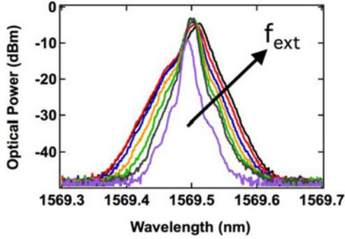
Fig. 2. Measured optical spectra of a 1.55- $\mu\text{m}$  InAs/InP QD DFB laser for various feedback levels  $f_{\text{ext}}$ . The last spectrum (black color) corresponds to the fully developed coherence collapse regime.
