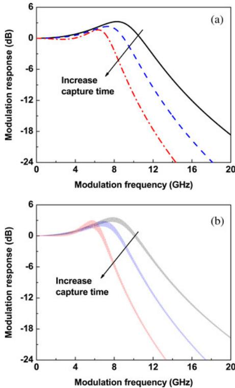
Fig. 8. Impacts of various carrier capture time  $0.2 \tau_{\text{ES}}^{\text{WL}}$ ,  $1.0 \tau_{\text{ES}}^{\text{WL}}$ , and  $2.0 \tau_{\text{ES}}^{\text{WL}}$  on the IM response for (a) short external cavity ( $f_{\text{ext}} = 10^{-3}$ , LEF = 1) and (b) long external cavity ( $f_{\text{ext}} = 10^{-5}$ , LEF = 5).
