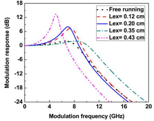
Fig. 6. Impacts of the feedback phase on the IM response for  $\tau_{\text{ES}}^{\text{WL}} = 0.5$  ps,  $\tau_{\text{GS}}^{\text{ES}} = 0.5$  ps,  $\alpha_H = 1$ ;  $f_{\text{ext}} = 10^{-2}$ ;  $L_{\text{ex}} = 0.12$  cm ( $\phi_0 = 2\pi \times 0.24$ );  $L_{\text{ex}} = 0.20$  cm; ( $\phi_0 = 2\pi \times 0.73$ );  $L_{\text{ex}} = 0.35$  cm ( $\phi_0 = 2\pi \times 0.02$ ); and  $L_{\text{ex}} = 0.43$  cm ( $\phi_0 = 2\pi \times 0.51$ ).
