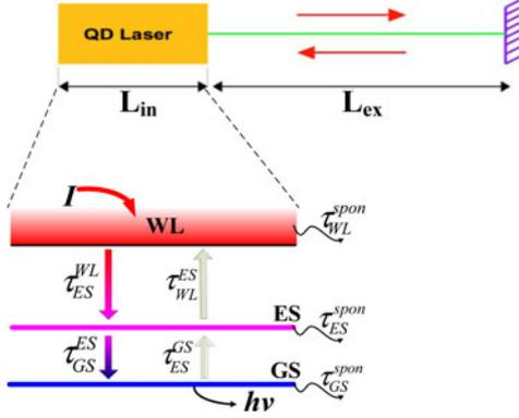
Fig. 1. Basic scheme of QD lasers operating under self-injection, and sketch of the corresponding carrier dynamics.
