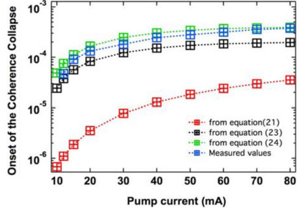
Fig. 3. Measured onset of the coherence collapse as a function of the pump current for a 1.55- $\mu\text{m}$  InAs/InP QD DFB laser (blue squares). Red, black, and green squares correspond to the extracted onset of the coherence collapse from (21), (23), and (24). Dotted lines are added for visual help only.
