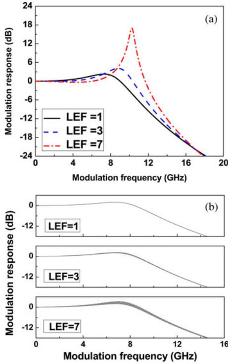
Fig. 7. Impacts of LEF on the IM response for (a) short external cavity ( $f_{\text{ext}} = 10^{-3}$ ) and (b) long external cavity ( $f_{\text{ext}} = 10^{-5}$ ).
