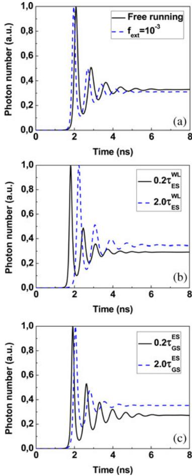
Fig. 10. TOD properties (a) without and with optical feedback ( $f_{\text{ext}} = 10^{-3}$ ) at  $\tau_{\text{ES}}^{\text{WL}} = 12.6$  ps and  $\tau_{\text{GS}}^{\text{ES}} = 5.8$  ps (b) for various capture times at  $0.2\tau_{\text{ES}}^{\text{WL}}$  and  $2\tau_{\text{ES}}^{\text{WL}}$  with  $f_{\text{ext}} = 10^{-3}$  and (c) for various relaxation times at  $0.2\tau_{\text{GS}}^{\text{ES}}$  and  $2\tau_{\text{GS}}^{\text{ES}}$  with  $f_{\text{ext}} = 10^{-3}$ .
