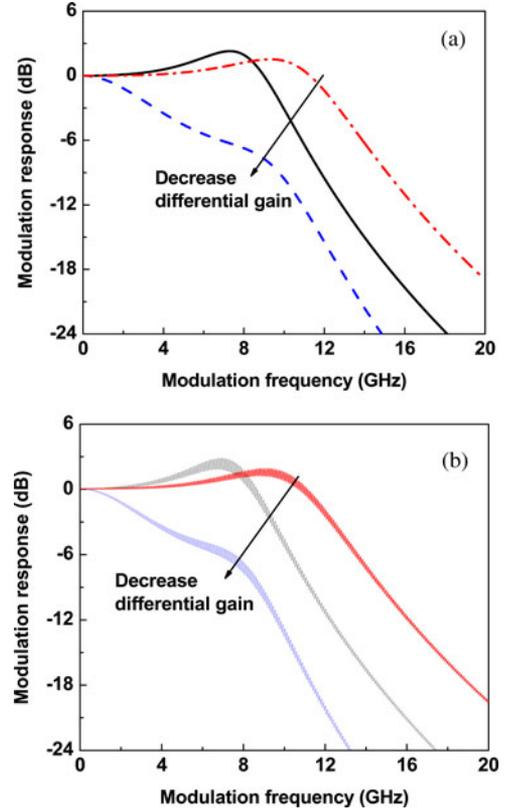
Fig. 11. Impacts of various differential gain  $a_{\text{GS}} = 3 \times 10^{-15}$ ,  $5 \times 10^{-15}$ , and  $10 \times 10^{-15}$  cm $^2$  on the IM response for (a) short external cavity ( $f_{\text{ext}} = 10^{-3}$ ) and (b) long external cavity ( $f_{\text{ext}} = 10^{-5}$ ).
