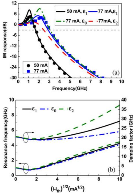
Fig. 12. (a) IM response for a free-running laser under various gain compression factor  $\epsilon_1 = 3 \times 10^{-16} \text{ cm}^3$ ,  $\epsilon_0 = 0$ , and  $\epsilon_2 = 9 \times 10^{-16} \text{ cm}^3$ . Dots represent experimental results and lines represent simulations. (b) Resonance frequency and damping factor as a function of the normalized current.
