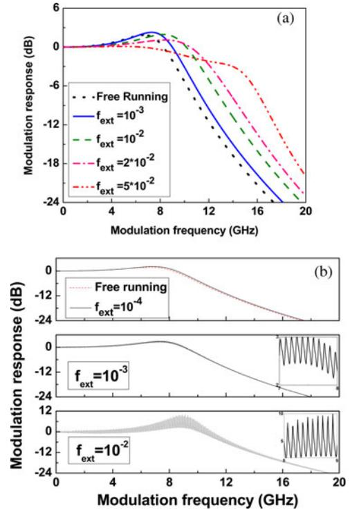
Fig. 4. Impacts of the feedback level on the IM response for (a) short external cavity and (b) long external cavity.
