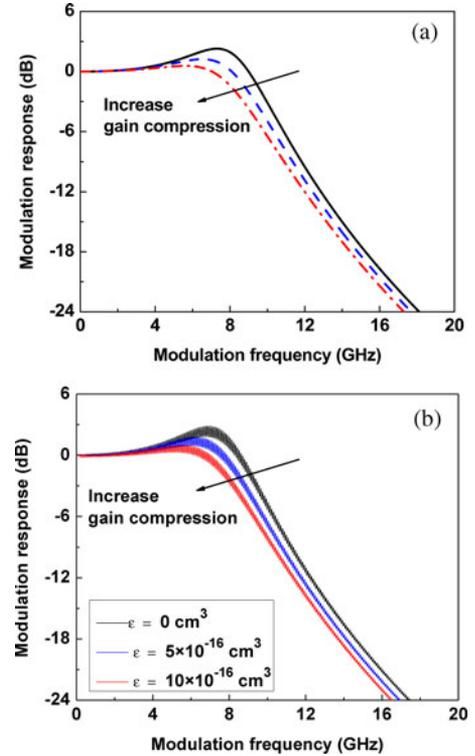
Fig. 13. Impacts of gain compression on the IM response with  $\epsilon = 0, 5 \times 10^{-16}, 10 \times 10^{-16} \text{ cm}^3$  for (a) short external cavity ( $f_{ext} = 10^{-3}$ ) and (b) long external cavity ( $f_{ext} = 10^{-5}$ ).
