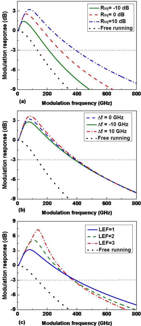
FIG. 4. IM response of optical injection-locked QCLs for slow carrier removal rate ( $\tau_R = 1.2$  ps) as a function of (a) injection ratio  $R_{inj}$  at zero detuning with  $LEF = 1$ , (b) detuning frequency  $\Delta f$  at  $R_{inj} = 10$  dB with  $LEF = 1$ , and (c)  $LEF$  at zero detuning with  $R_{inj} = 10$  dB.
