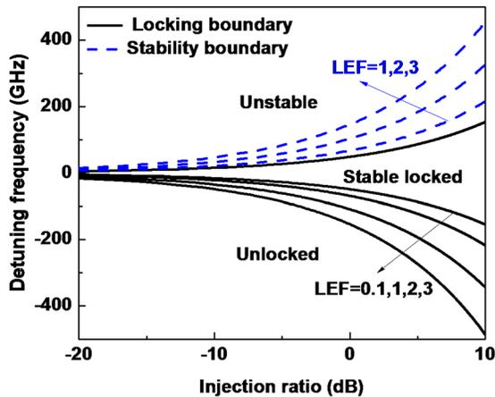
FIG. 2. Optical injection-locking diagram as function of the detuning frequency and the injection ratio. Solid lines are the locking regime boundaries; the negative detuning frequency boundaries are calculated with LEF = 0.1, 1, 2, and 3, respectively; dashed line is the stability boundary.
