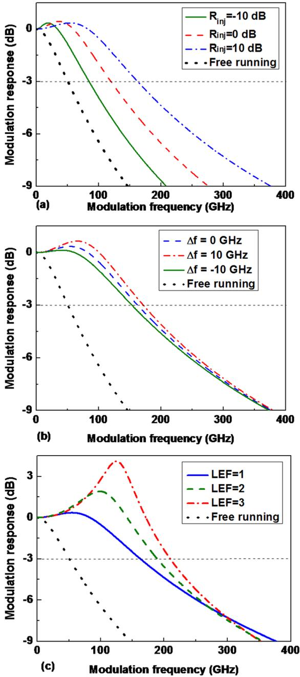
FIG. 3. IM response of optical injection-locked QCLs for fast carrier removal rate ( $\tau_R = 0.21$  ps) as a function of (a) injection ratio  $R_{inj}$  at zero detuning with  $LEF = 1$ , (b) detuning frequency  $\Delta f$  at  $R_{inj} = 10$  dB with  $LEF = 1$ , and (c)  $LEF$  at zero detuning with  $R_{inj} = 10$  dB.
