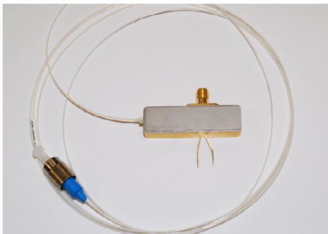
Fig. 2. Picture of the passive QDMLL packaged module. The RF connector shown on the top of the package was not used for this experiment.
