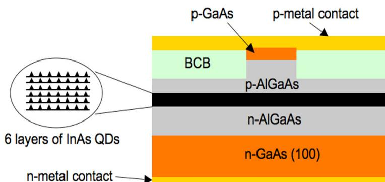
Fig. 1. Schematic of the epitaxial layer structure of the InAs QD laser.
