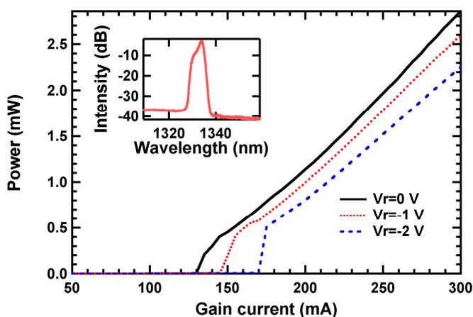
Fig. 3. L-I characteristics measured at 20°C under various absorber biases. Inset: the optical spectrum under 280-mA gain current and -1 V reverse voltage.
