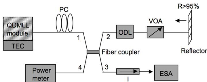
Fig. 4. Schematic drawing of the experimental setup. PC: polarization controller; ODL: optical delay line; VOA: variable optical attenuator; I: isolator; ESA: electrical spectrum analyzer.
