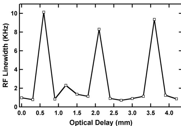
Fig. 5. RF linewidth variation under feedback ratio of -44 dB as a function of optical delay line change at 20°C, showing a periodicity of roughly 1.5 mm corresponding to the laser round trip time of 200 ps. Bias condition of QD MLL: 280 mA gain current and -1 V reverse voltage.
