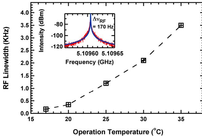
Fig. 6. Evolution of RF linewidth versus operation temperature under optimized external optical feedback. Inset: RF linewidth of 170 Hz at 17°C under a feedback ratio as low as -42 dB.
