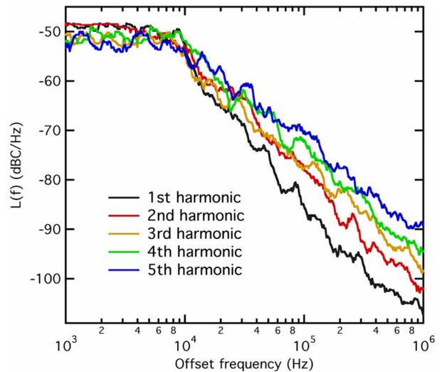
Fig. 8. SSB-PN spectra density from different harmonics under 100-mA gain current and  $-7$ -V reverse voltage at the optimum feedback case.
