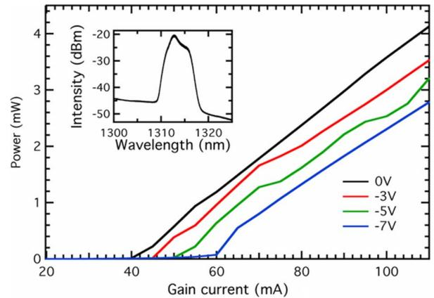
Fig. 2. Light current characteristics measured at  $20^\circ\text{C}$  under various absorber bias voltages. The figure in the inset shows the optical spectrum under 280-mA gain current and  $-1\text{ V}$  reverse voltage.
