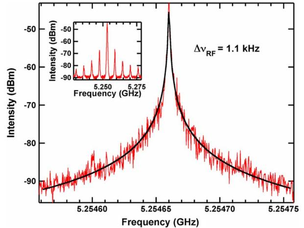
Fig. 7. RF linewidth of 1.1 kHz under optimum feedback condition ( $\Gamma = -33$  dB). Inset: RF spectrum with mode-comb separated by 5.7 MHz.
