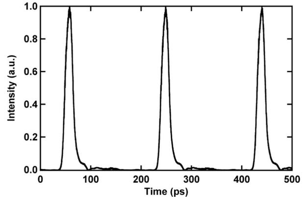
Fig. 3. Pulse width of 10.9 ps under 75-mA gain current and  $-7\text{ V}$  reverse voltage through high-speed sampling oscilloscope measurement.
