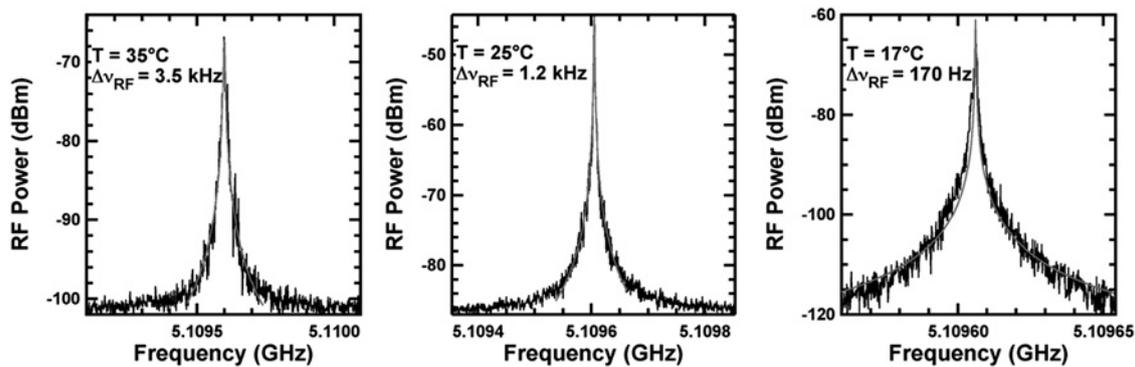
**Fig. 6** Evolution of the RF linewidth for three different temperatures under the stably resonant feedback condition
