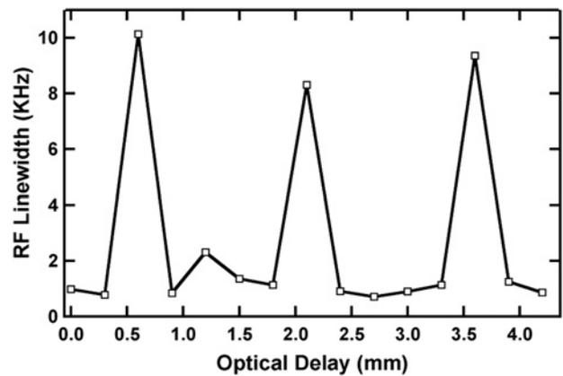
**Fig. 5** RF linewidth variation under feedback ratio of  $-44\text{ dB}$  as a function of optical delay line change at  $20^\circ\text{C}$ , showing a periodicity of roughly 1.5 mm corresponding to the laser round trip time of 200 ps
