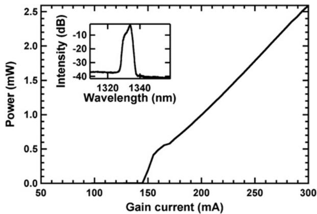
**Fig. 3**  $L$ - $I$  characteristic measured at  $20^\circ\text{C}$  for an absorber bias of  $-1\text{ V}$
