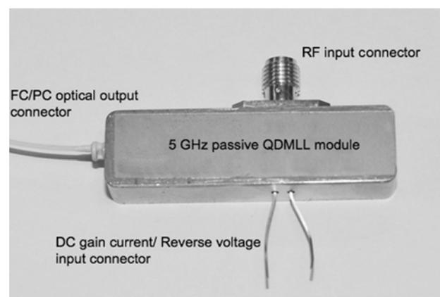
**Fig. 2** Picture of the passive QD MLL packaged module
