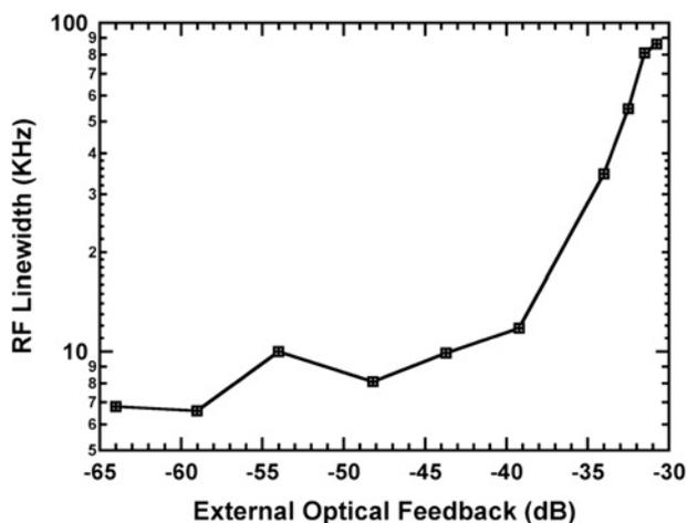
**Fig. 7** RF linewidth as a function of the external feedback ratio at a bias of 280 mA gain current and  $-1$  V on the absorber at 20°C under nearly exact resonant case
