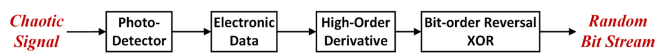
FIG. 12. Schematic diagram of the processes implemented in order to produce random bits with the experimental hyperchaos generated by the solitary ICL.
