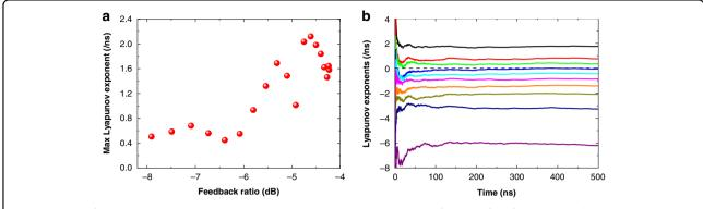
Fig. 3 Analysis of the Lyapunov exponents at 85 mA. a Largest Lyapunov exponent as a function of the feedback ratio. b Lyapunov spectrum at the feedback ratio of -4.2 dB.
