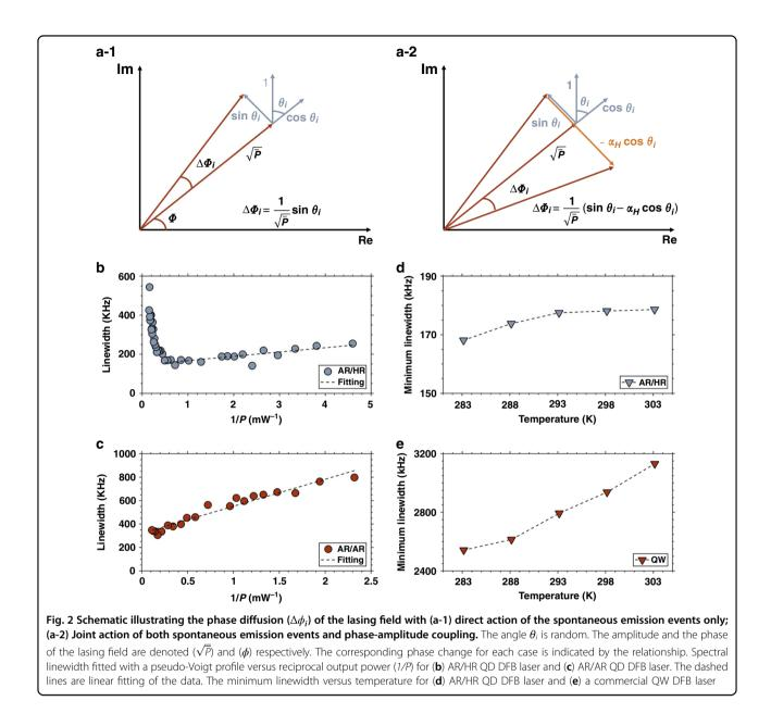
contributed from the spontaneous emission events and the phase-amplitude coupling effect, which is described by the  $\alpha_{H}$ -factor, associated to the interaction between the intensity and phase of the lasing field. Consequently, the spectral linewidth of a semiconductor laser can be retrieved from the mean-square of the phase jitter. The corresponding equation known as the extended Schawlow-Townes relationship as follows<sup>53</sup>:
