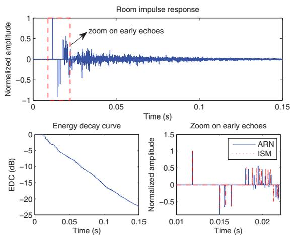
Figure 4: Simulation results of Room 2 with absorption  $\alpha = 0.25$ .
