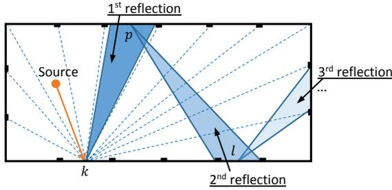
Figure 1: Illustration of discretized specular reflections.
