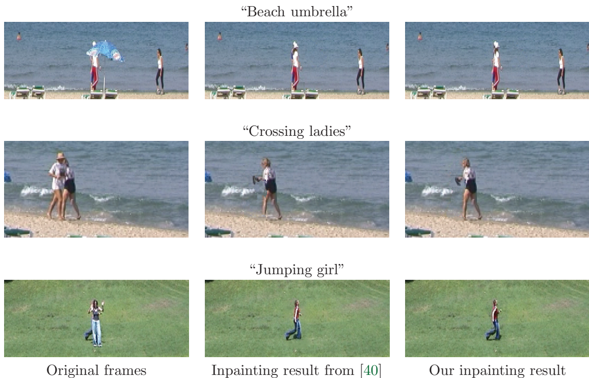
Figure 8. Comparison with Wexler, Shechtman, and Irani. We achieve results of similar visual quality to those in [40], with a reduction of the ANN search time by a factor of up to 50 times. [Image credits: http://www.wisdom.weizmann.ac.il/~vision/VideoCompletion.html .]
