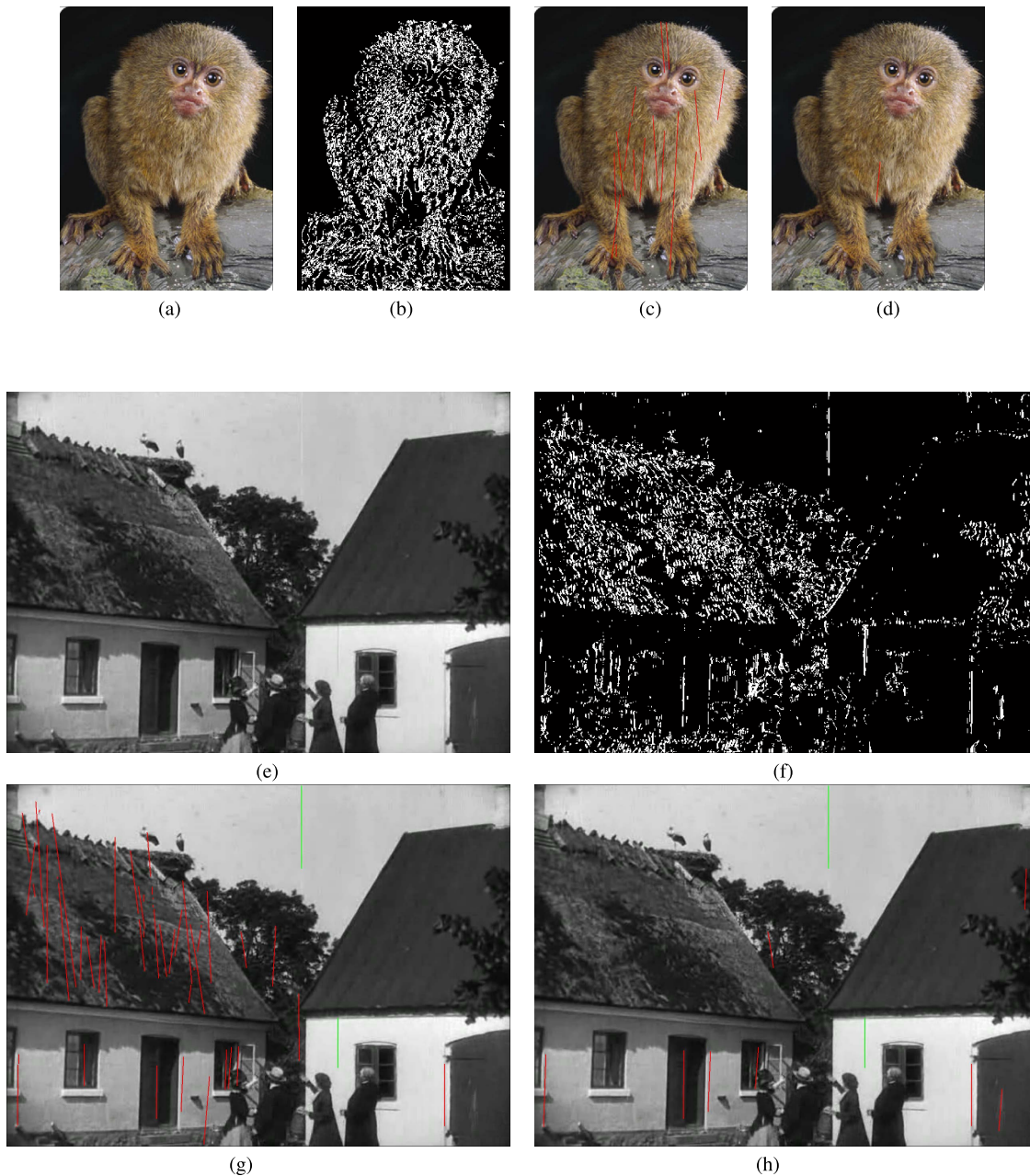
Fig. 8. An illustration of our spatial method's robustness to texture and noise on two highly textured test images. In the first example, our locally adaptive method produces only one false detection, whereas with a global background model estimation, the algorithm fails. The second example illustrates this principle on an image with real scratches. (a) Original frame. (b) Binary detection. (c) A contrario detection with a global background model estimation. (d) A contrario detection with a local background model estimation. (e) Original frame. (f) Binary detection image. (g) A contrario detection with a global background model estimation. (h) A contrario detection with a local background model estimation.
