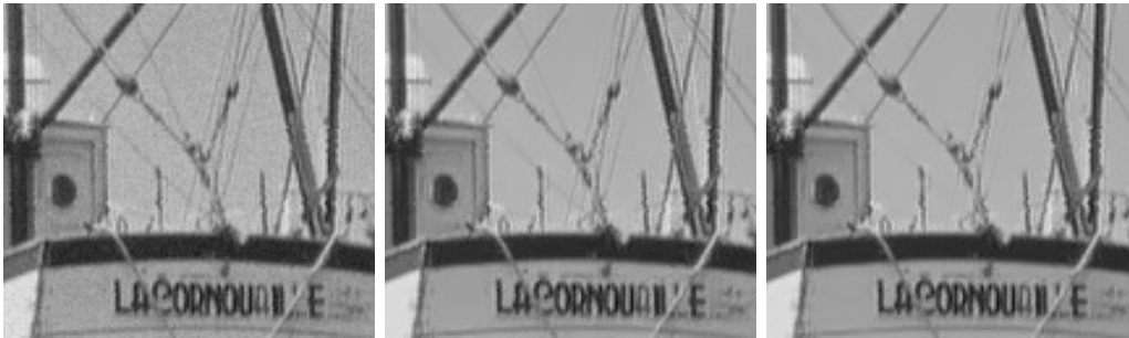
Figure 2. Loss of lines and isolated details. Left: boat image with little noise ( \sigma = 5 ). Middle: result of the NLM filter ( h = 6 , s^2 = 7 \times 7 , search window 11 \times 11 ). Right: same experiment, using a search window 61 \times 61 . Notice that several ropes vanish when the size of the search window increases (this should be seen on a computer screen).
