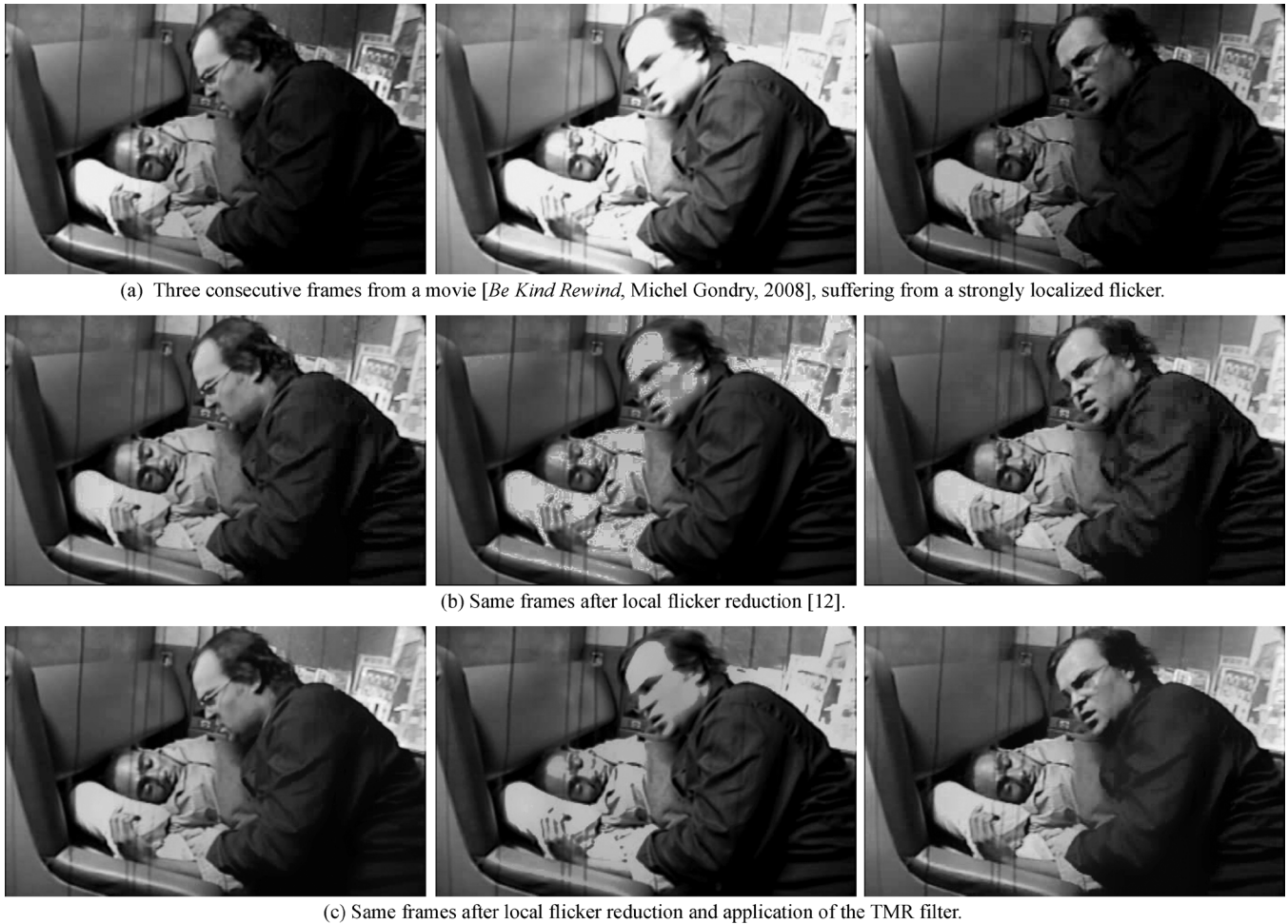
Fig. 5. Application of the iterated TMR filter to flicker stabilization. (a) Sequence of three images corrupted by flicker (strong and fast local contrast change). (b) Flicker stabilization results with the method of Delon and Desolneux [12]. Observe that the contrast is well harmonized over the sequence, but some artefacts related to brutal and local contrast modifications appear. (c) Same frames after local flicker reduction and application of the TMR filter. Iterated TMR filter permits to remove those artefacts.
