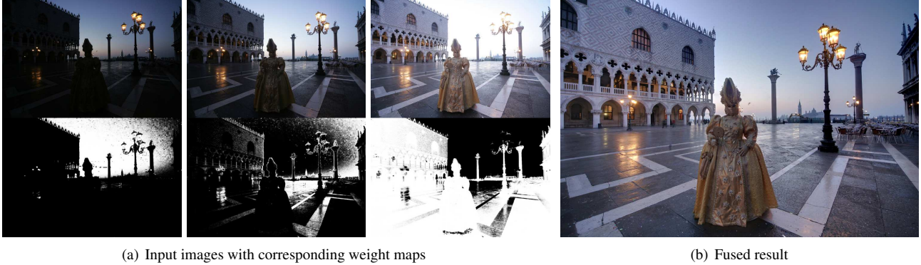
Figure 2. Exposure fusion is guided by weight maps for each input image. A high weight means that a pixel should appear in the final image. These weights reflect desired image qualities, such as high contrast and saturation. Image courtesy of Jacques Joffre.
