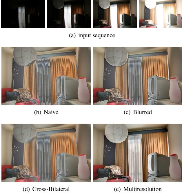
Figure 4. Weighted blending. The input sequence is shown in (a). Naive per-pixel blending (b) yields obvious seams due to sharp variations in the weight map. Blurring the weight map using a Gaussian kernel (c) removes the seams, but introduces halos around edges. Cross-bilateral filtering (d) is able to avoid some of the halos, but not all. Multiresolution blending (e) creates the desired result.
