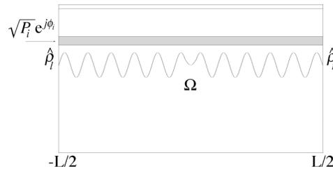
Fig. 1. Phase-shifted index-coupled DFB laser heterostructure.
