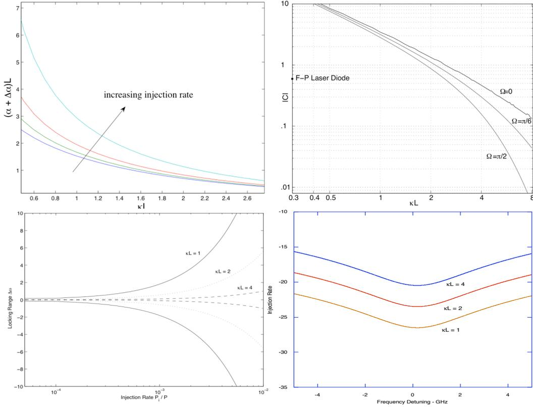
Fig. 2. (a) Threshold gain in the free running regime (lower curve) and its modification due to injection. (b) Coefficient  $C$  dependence on the coupling strength for various phase shifts. (c) Static locking range and (d) static/dynamic limit.
