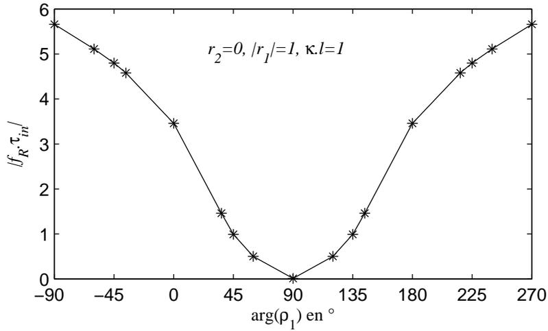
**Figure 3.** Feed-in rate for backward injection in function of the rear facet phase for a AR/HR DFB laser
