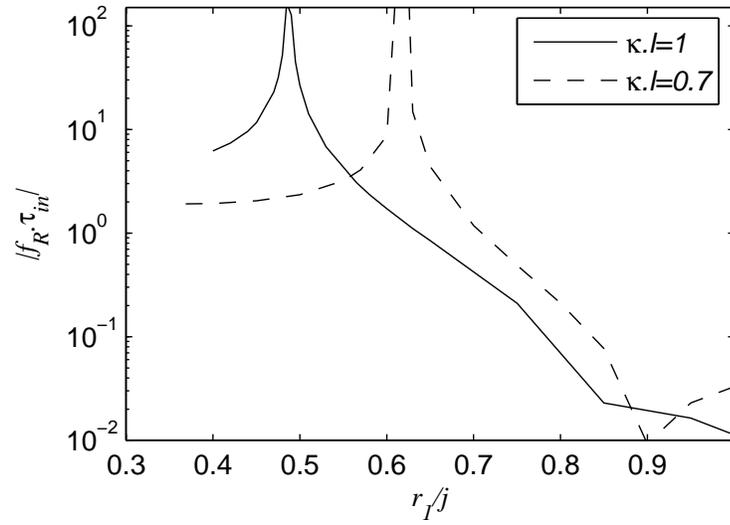
**Figure 4.** Feed-in rate for backward injection in function of the rear facet reflectivity for gap mode DFB laser
