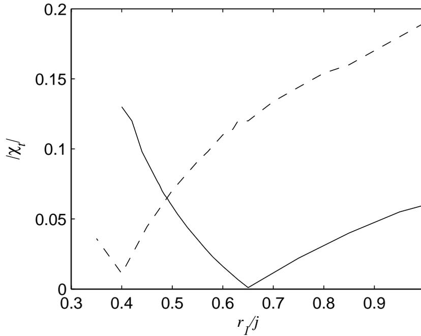
**Figure 6.** Module of  $\chi_t$  parameter for forward injection in function of the rear facet reflectivity for gap mode DFB laser
