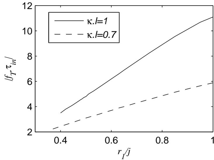
**Figure 5.** Feed-in rate for forward injection in function of the rear facet reflectivity for gap mode DFB laser
