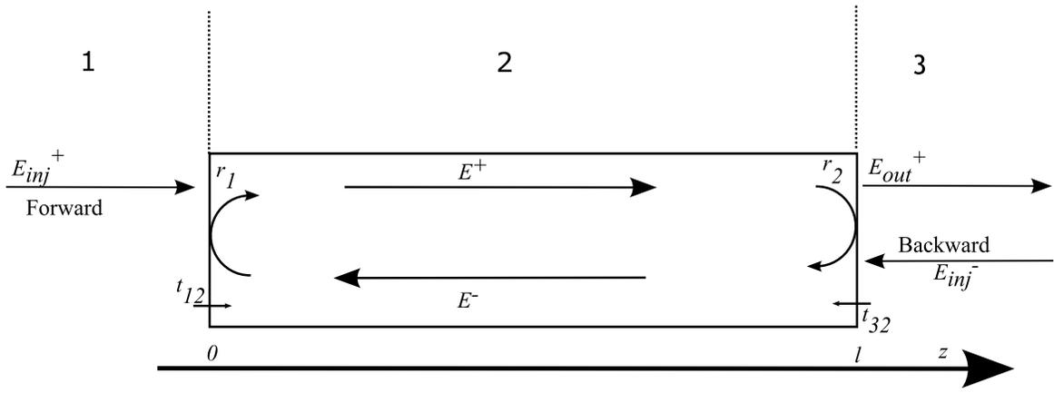
Figure 1. Forward and backward injection in a laser
