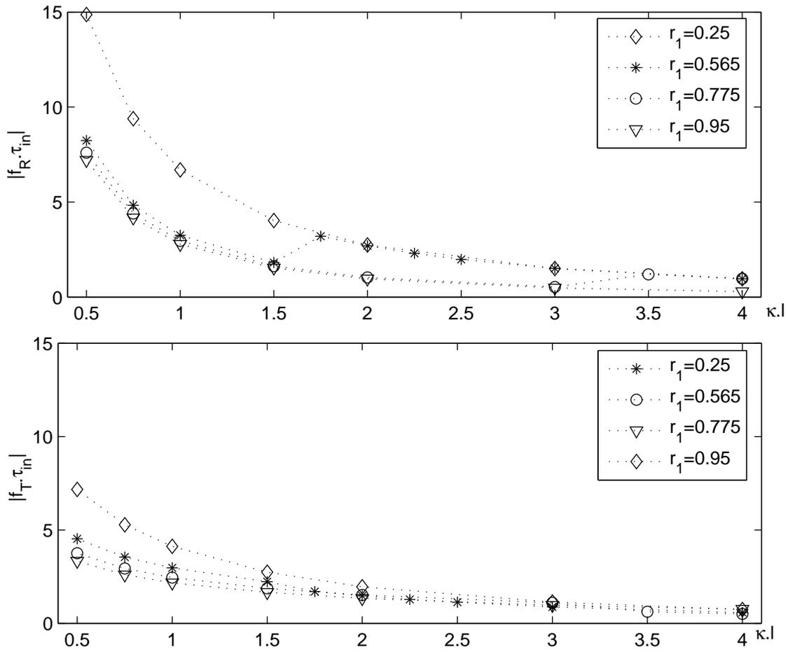
**Figure 2.** Feed-in rate for backward and forward injection in function of the grating coupling factor for different reflectivity values of the left facet
