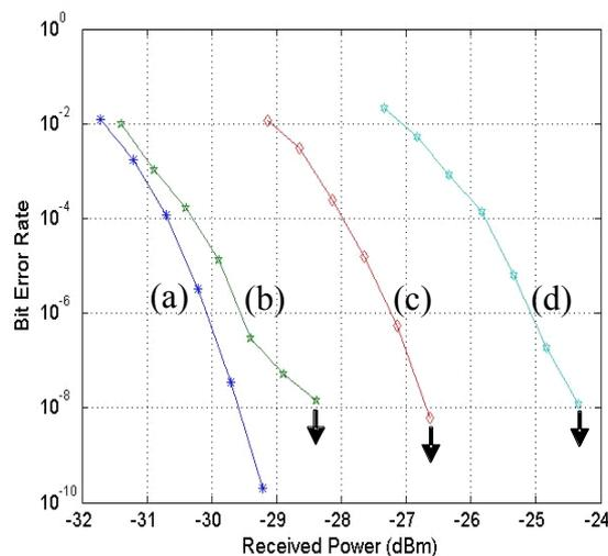
**Figure 5.** BER measurements vs. received optical power: (a) back to back (i.e. without encoder/decoder), (b) single user case, (c) two users asynchronous case and (d) two users synchronous case.
