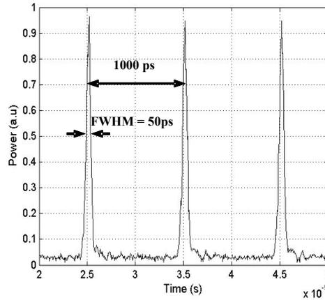
**Figure 4.** Waveform of RZ optical pulse train generated by the first stage at 1/10 repetition rate.
