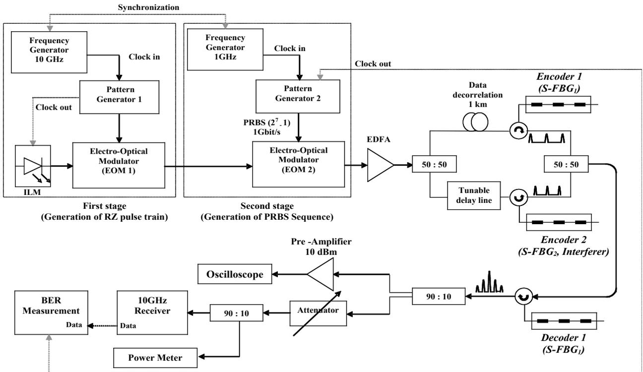
**Figure 3.** Experimental setup of BER measurement involving 2 multiplexed users.
