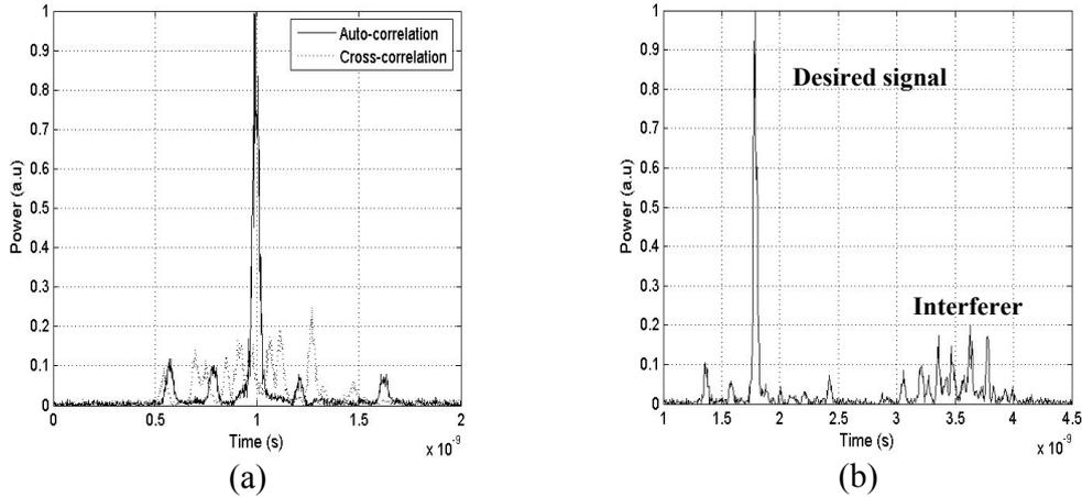
**Figure 2.** Measured auto and cross-correlation function: (a) Single-user configuration (without interferer), (b) Two-users configuration (in presence of one interferer).
