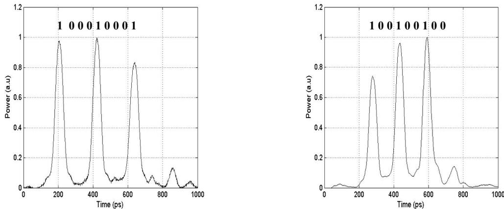
**Figure 1.** Prime Sequence codewords  $C_1$  and  $C_2$  generated by S-FBG<sub>1</sub> and S-FBG<sub>2</sub>
