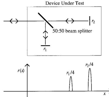
Fig. 3. Physically separated light paths in the device under test.
