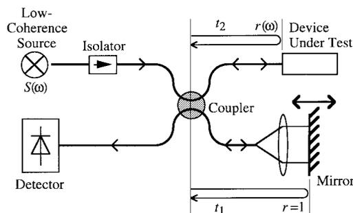
Fig. 1. Simplified schematic diagram of the optical low-coherence reflectometer.
