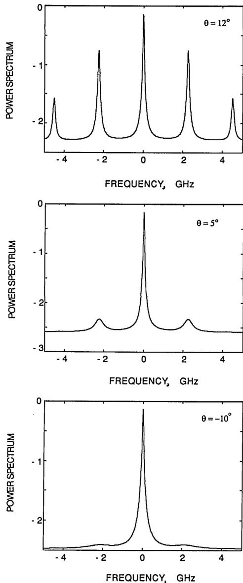
Fig. 2. Power spectra: logarithmic relative intensity versus the frequency for an output power of the locked laser of 2 mW, an output power of the master laser of 4 mW, and an injection level  $P_i/P$  of  $-30$  dB for different values of the phase detuning  $\theta$ .
