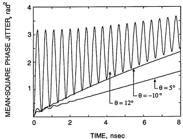
Fig. 1. Mean-square phase jitter  $\langle \Delta\varphi^2(\tau) \rangle$  of the locked laser:  $\langle \Delta\varphi^2(\tau) \rangle$  versus time  $\tau$  at an output power of 2 mW for the locked laser, an output power of 4 mW for the master laser, and an injection level  $P_i/P$  of -30 dB for different values of the phase detuning  $\theta$ .
